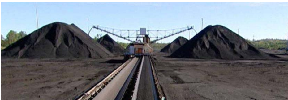
Figure B-13 Example of open dry bulk storage and transport by conveyor belt (Ref. [8])
