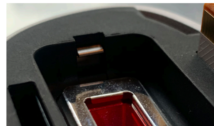
Figure 3.1.2; contamination sensitive splitlines and corners
