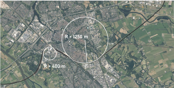
▲ 3.9 Train tracks near the station of Zwolle with radii between 400 m and 1250 m. Data: PDOK. Image: author
