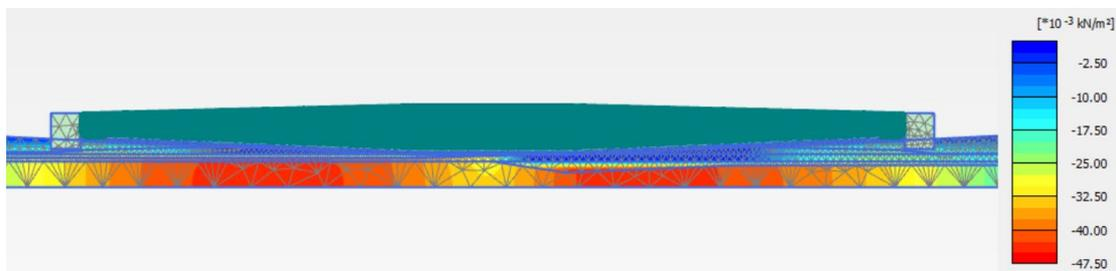
**Figure 6.10:** Excess pore water pressure under the loading of sand foundation
