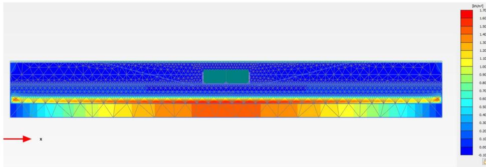
**Figure 5.9:** Excess pore water pressure due to reduce in tidal level
