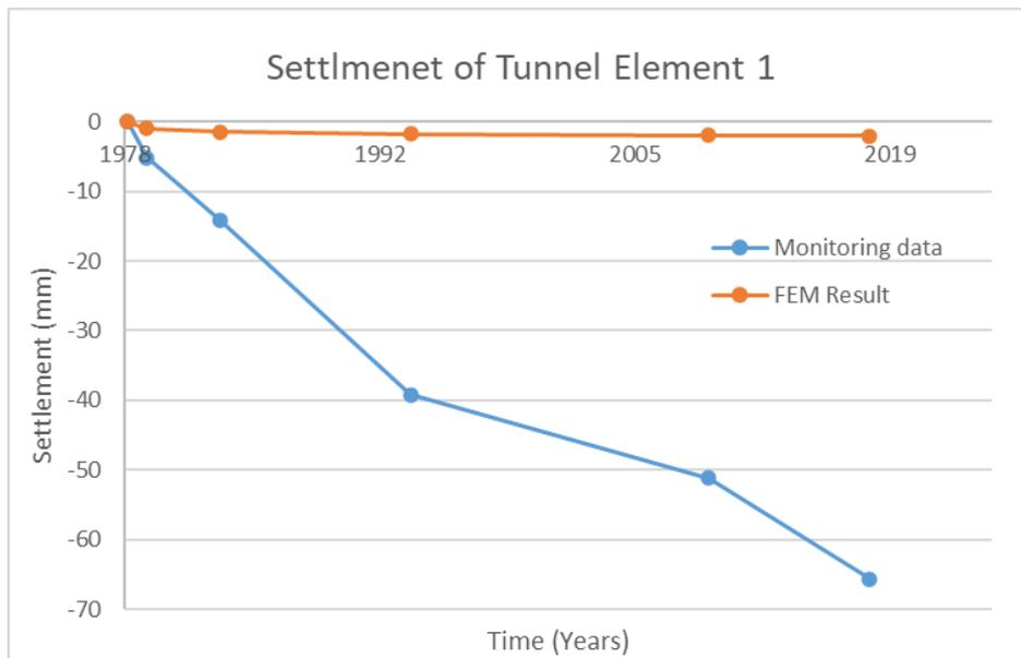
**Figure 4.17:** Comparison between monitoring data and FEM result
