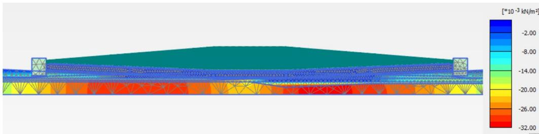
**Figure 6.22:** The excess pore water distribution
