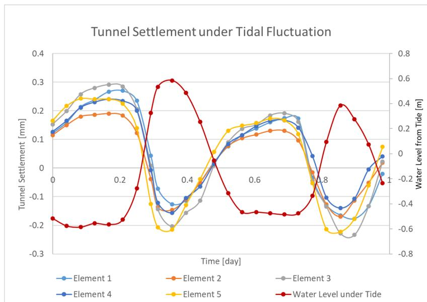
**Figure 5.15:** Settlement of immersed tunnel under two complete cycles of tide
