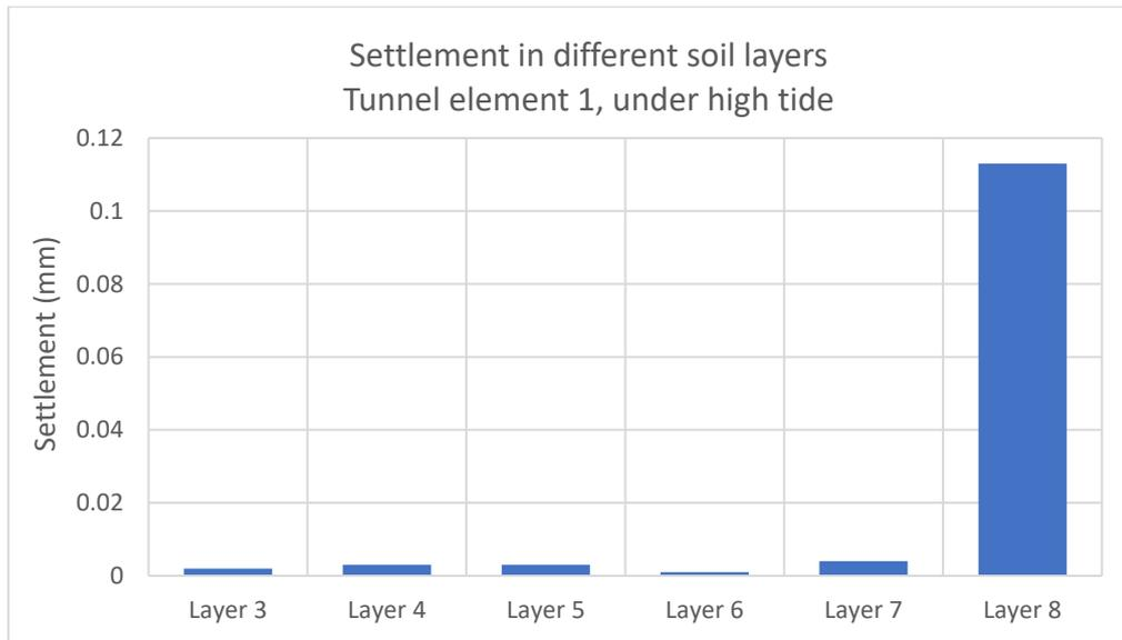
**Figure 7.9:** Histogram of soil settlement from tunnel element 1 under tidal fluctuation
