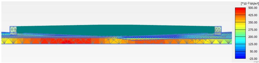
**Figure 6.8:** Excess pore water pressure distribution under trench excavation
