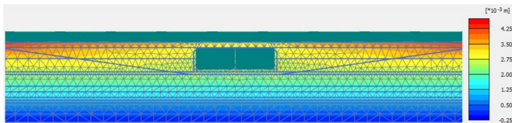
**Figure 5.7:** The rebounding of soil domain with 10kN/m unloading
