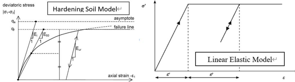
Figure 4.1: The stress and strain relationship of hardening soil and linear-elastic model
