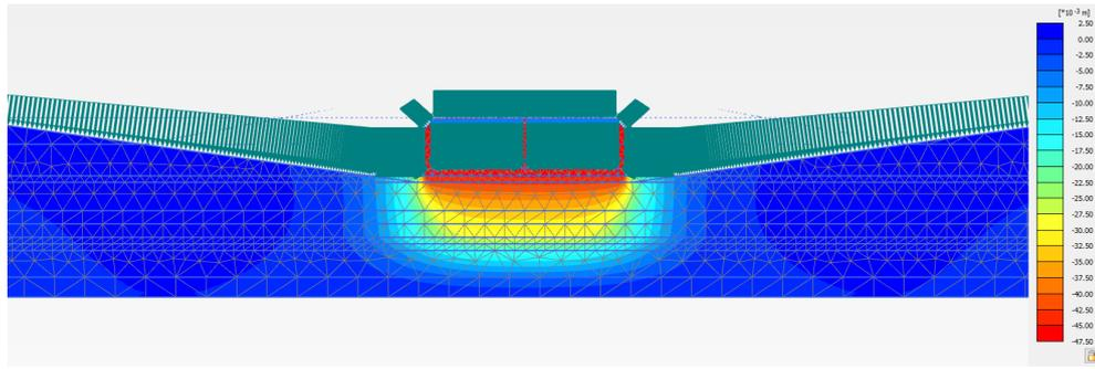
**Figure 4.10:** The settlement result from immersed tunnel construction
