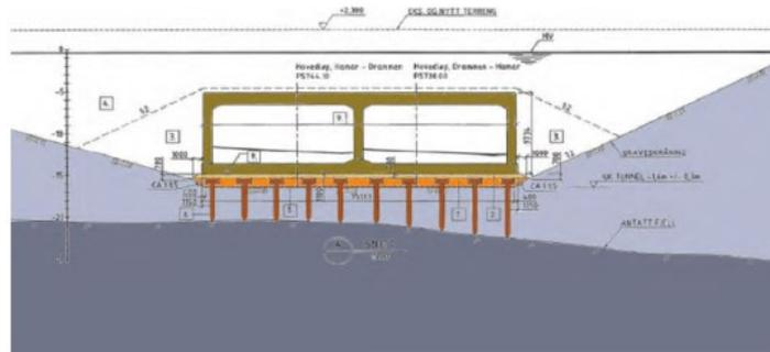
Figure 2.6: Cross Section of immersed tunnel that is supported by end bearing pile
