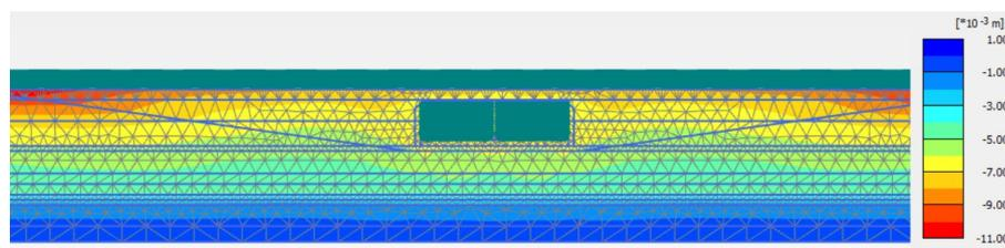
**Figure 5.6:** Settlement of immersed tunnel under pre-loading condition
