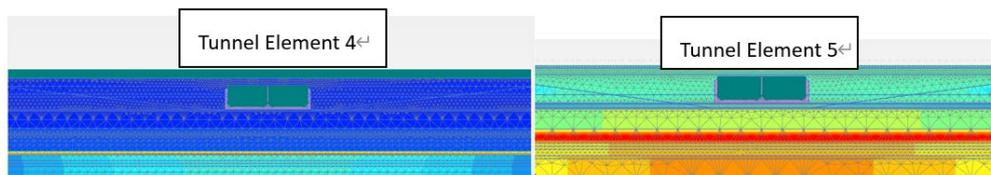
Figure 7.6: Excess pore water pressure distribution under high tidal condition
