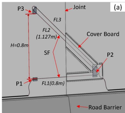
Figure 1.3: DOFS sensor at dilation joint in Heinenoordtunnel (Zhang and Wout, 2022)
