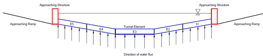
**Figure 6.2:** The hydraulic response of Heneoord tunnel under tide
