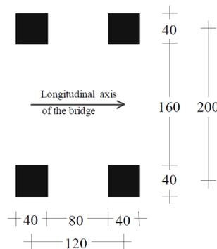
**Figure 4.20:** The tandem system on Load
