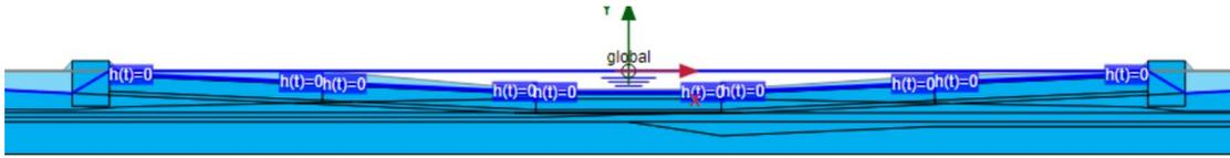
**Figure 6.4:** Water boundary condition of soil domain under the impact of tide
