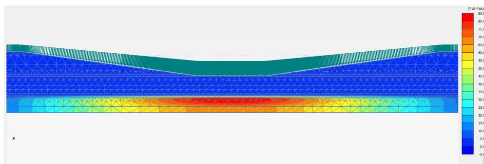
**Figure 4.9:** The excess pore water pressure distribution under trench excavation
