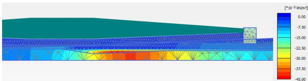
**Figure 6.20:** Excess pore pressure (0.044kPa) due to installation of tunnel element 4
