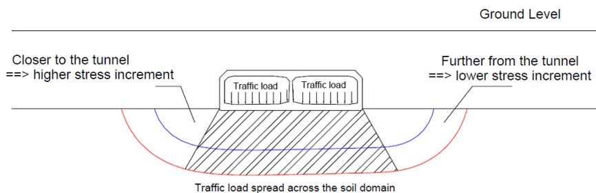
**Figure 7.4:** The load spread across the soil domain under different zone
