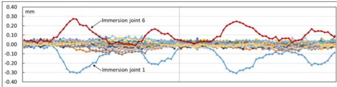
**Figure 1.4:** Daily uneven settlement behavior of immersion and dilation joint
