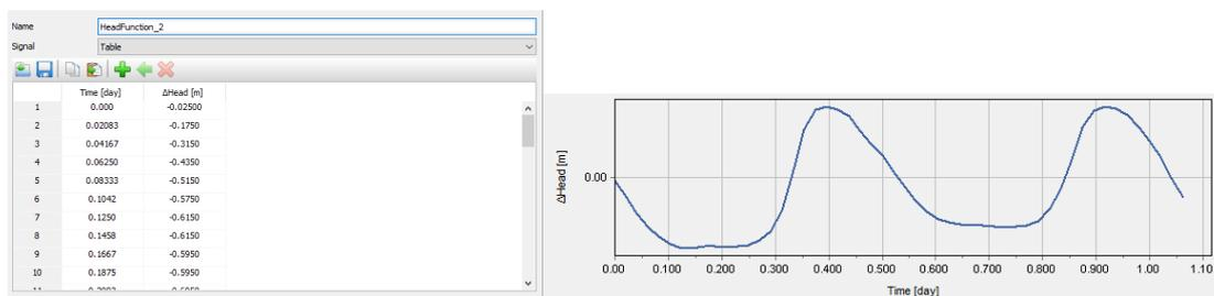
Figure 5.2: The input of water head (left) and the head function applied on Plaxis (right)
