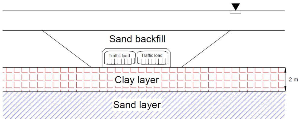
Figure 4.28: Simplified geological profile on creep settlement calculation
