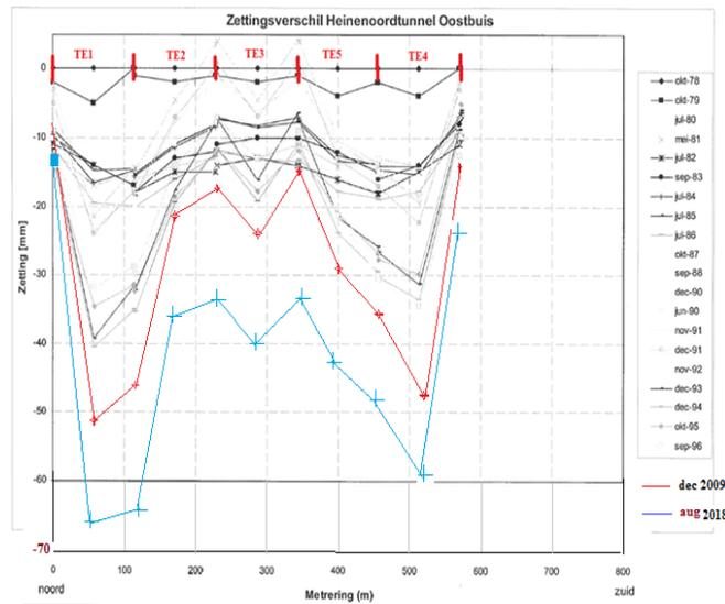
**Figure 4.16:** Monitoring result of Heinenoord tunnel from 1978 to 2018
