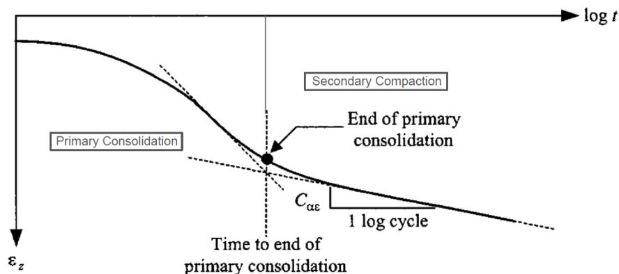
**Figure 4.27:** The time dependent behavior of NC clay under oedometer compaction
