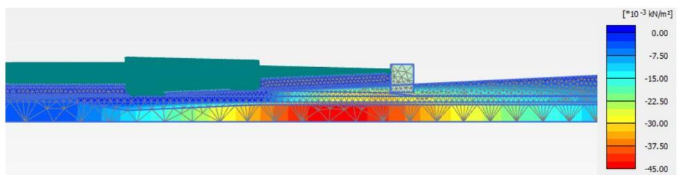
**Figure 6.19:** Excess pore pressure (0.044kPa) due to installation of tunnel element 5
