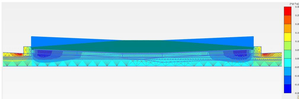
Figure 6.29: Settlement of immersed tunnel under the crest of the tide
