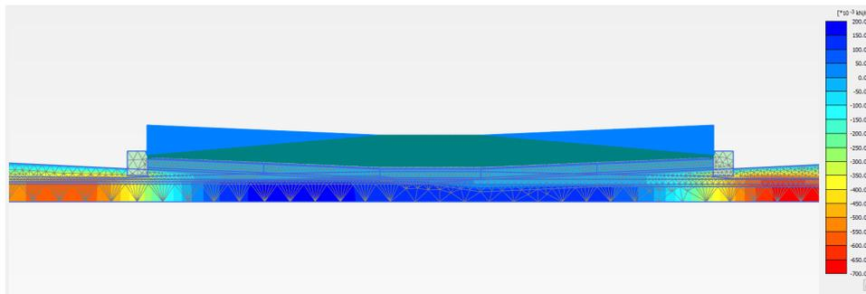
**Figure 6.34:** Excess pore water pressure distribution under the trough of the tide
