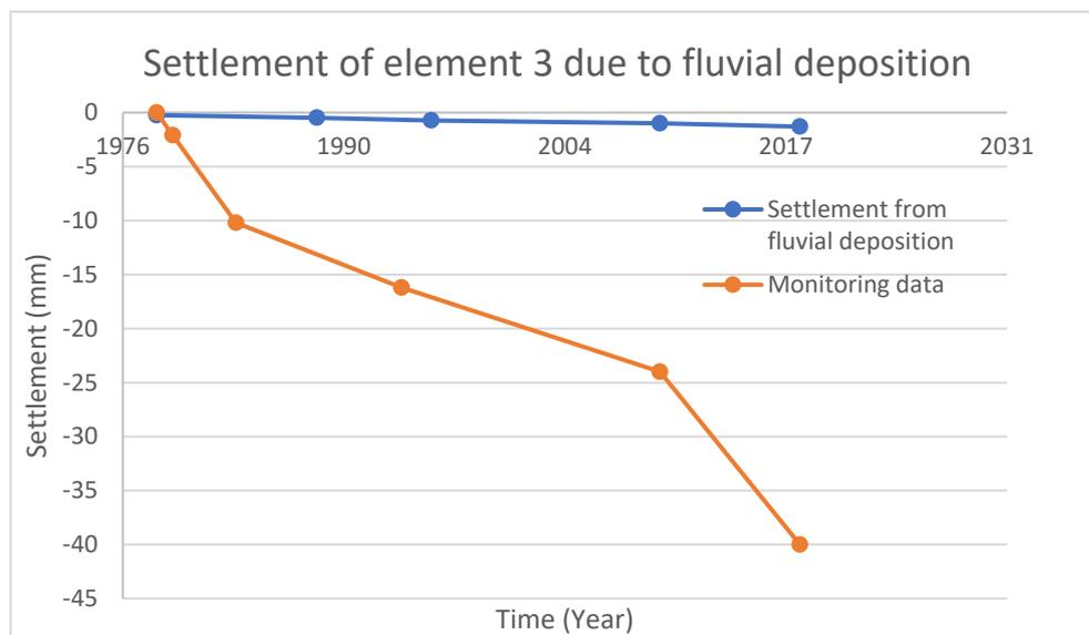
**Figure 4.26:** Result on settlement from fluvial depostion
