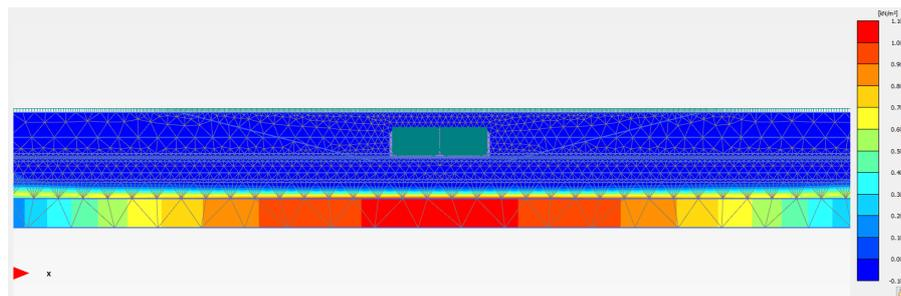
**Figure 5.11:** Excess pore water pressure under average water level
