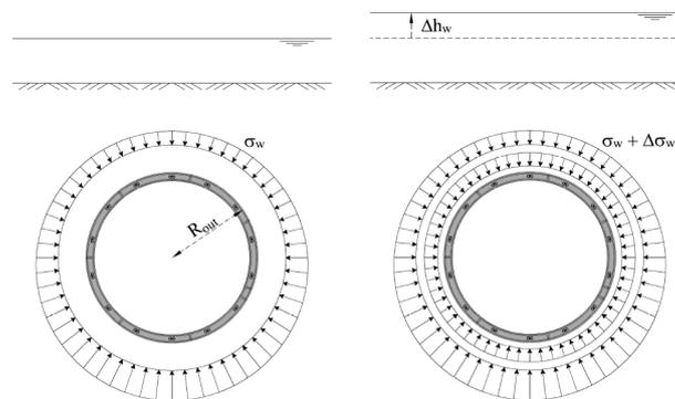
Figure 2.10 Tide induces hydrostatic stress on tunnel lining
