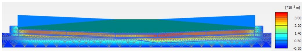
Figure 6.27: Rebound of Heinenoord tunnel under reloading of 10kN/m
