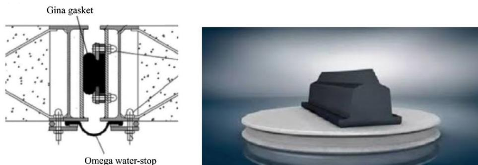
Figure 2.2: The detailing of immersion joint and the diagram of gina gasket
