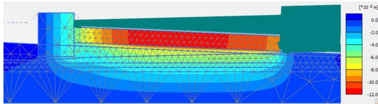
**Figure 6.11:** Settlement (1.16 cm) due to the installation of tunnel element 1
