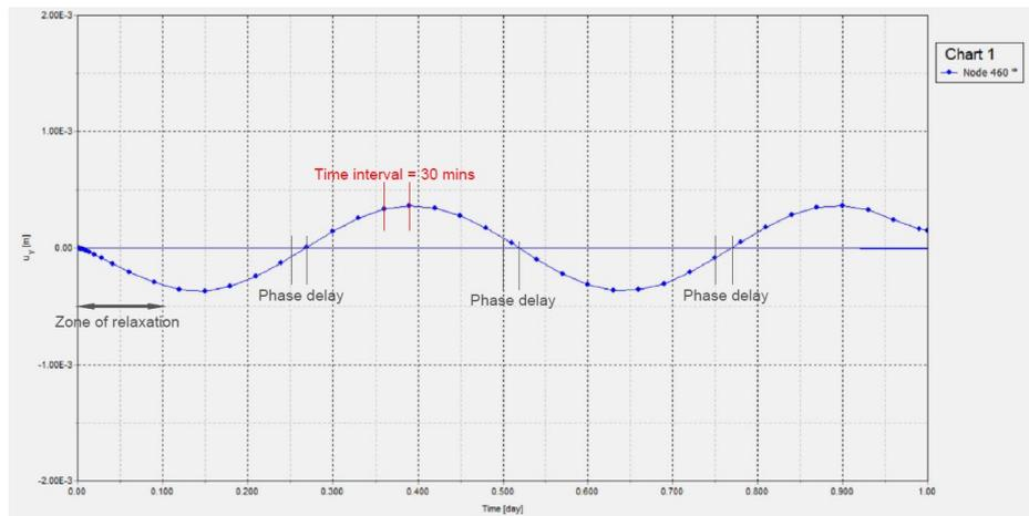
Figure 5.22: Settlement graph under the harmonic water boundary condition
