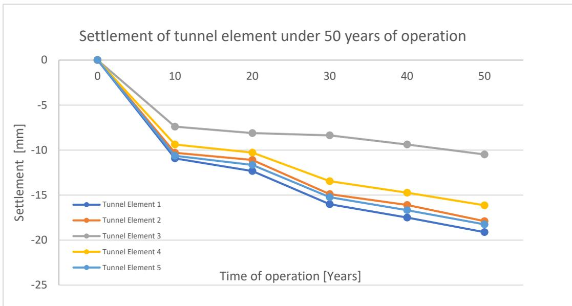
**Figure 6.25:** Settlement graph of tunnel element over the past 50 years of operation
