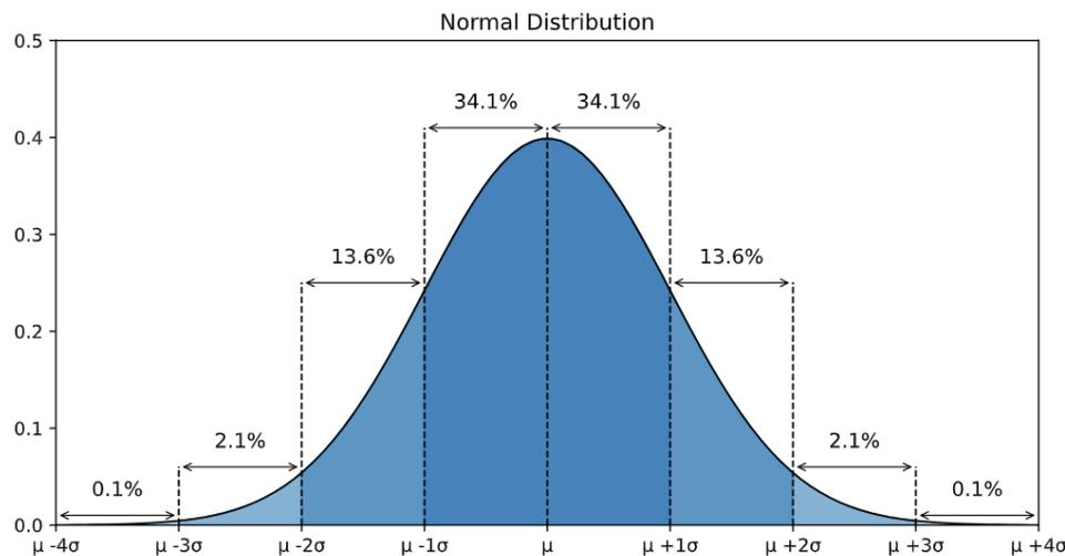
**Figure 7.3:** The probability density function under normal distribution
