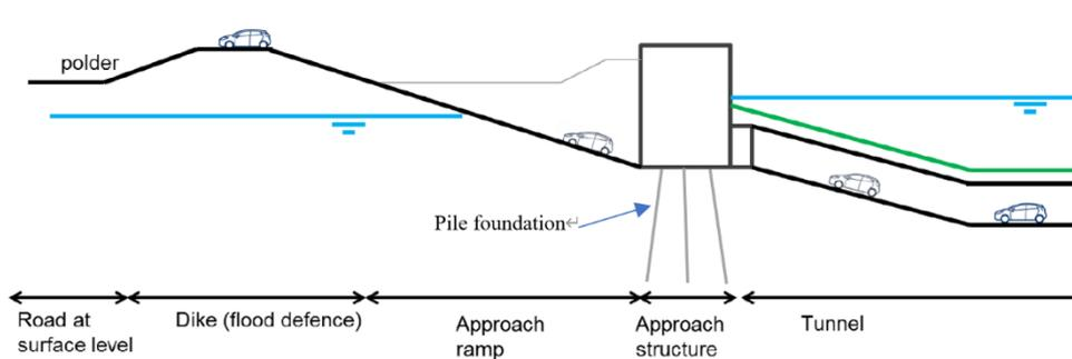
Figure 5.18: The longitudinal section of immersed tunnel and approaching structure
