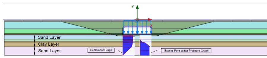
**Figure 5.14:** Behavior of soil under high tide condition
