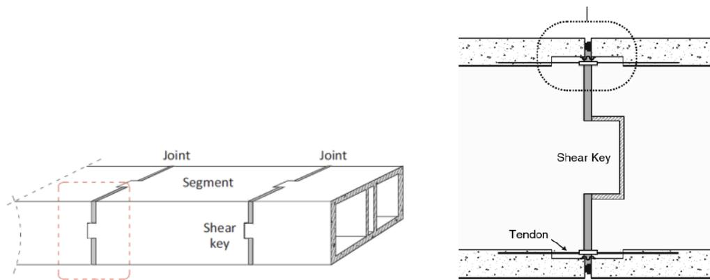
Figure 2.1: The detailing of segment joint in the global and local view
