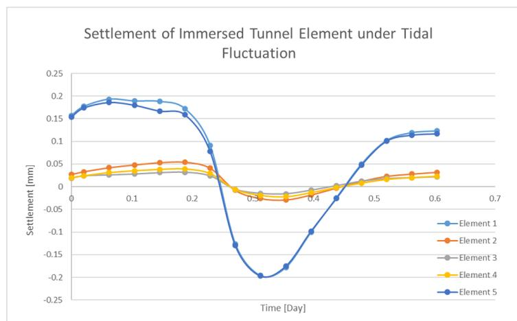
**Figure 6.35:** Settlement of tunnel element across time
