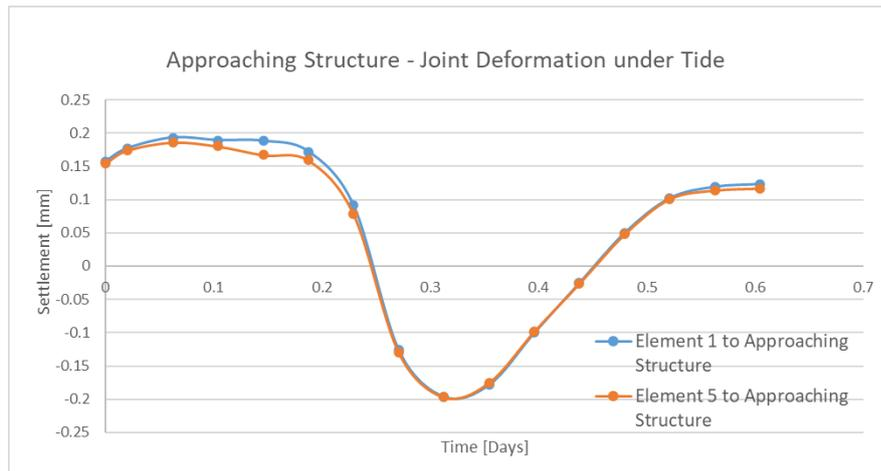
**Figure 6.37:** Joint deformation graph between approaching structure and element under tide
