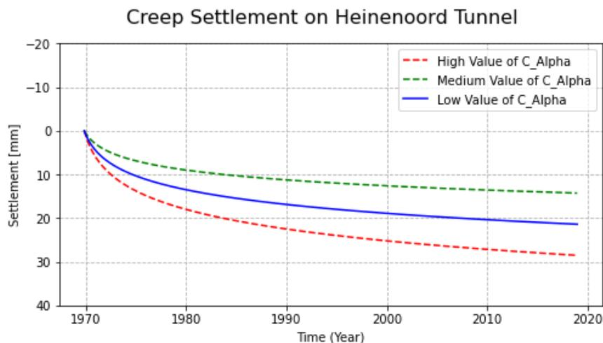
Figure 4.29: Creep settlement result on Heinenoord tunnel
