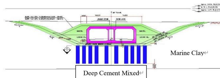
Figure 2.5: Cross Section of DCM in the ground treatment of immersed tunnel
