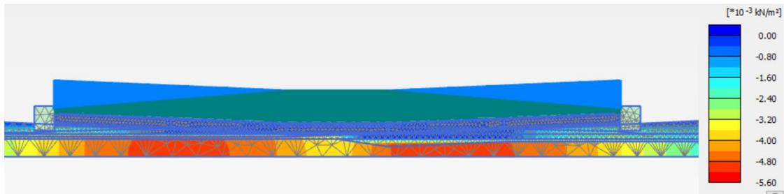
**Figure 6.24:** Excess pore water pressure of Heinenoord tunnel after 10 years of operation
