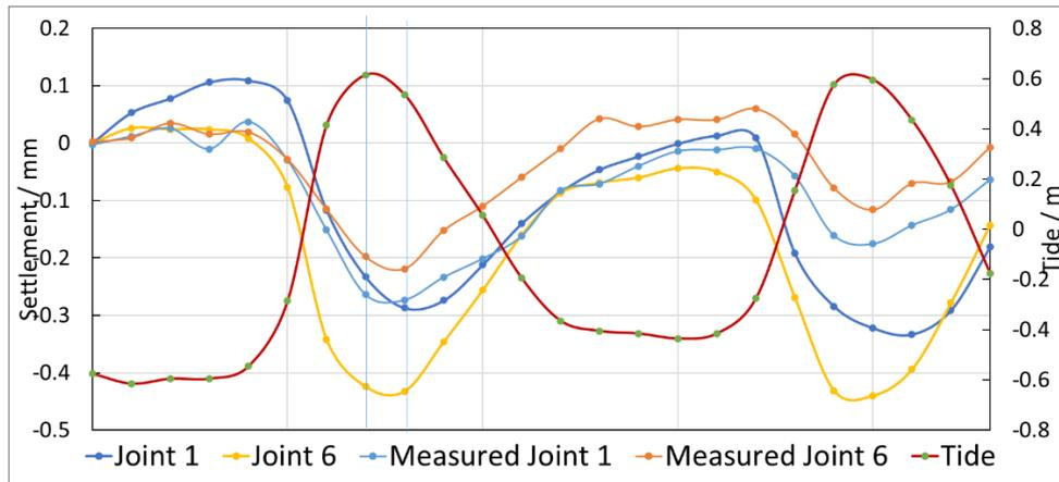
Figure 5.20: Immersion joint deformation between element and approaching structure
