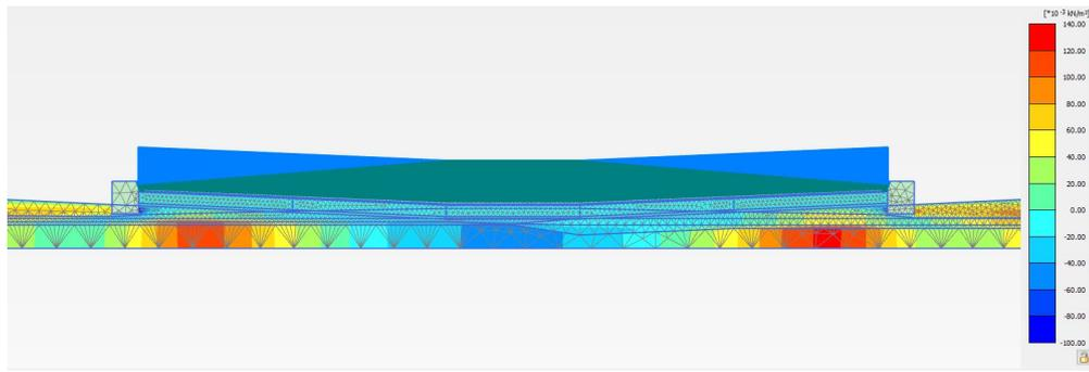
**Figure 6.32:** Excess pore water pressure of soil under mean water level
