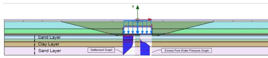
Figure 7.7: The excess pore water pressure and settlement under high tide events
