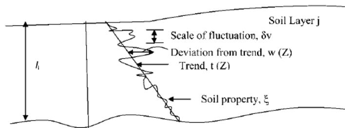
**Figure 7.2:** Variation of stiffness parameter with depth by Phoon and Kullhawy(1999)
