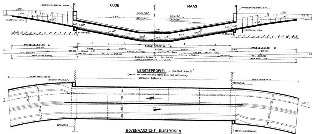
Figure 1.1: Longitudinal tunnel profile of Heinenoordtunnel
