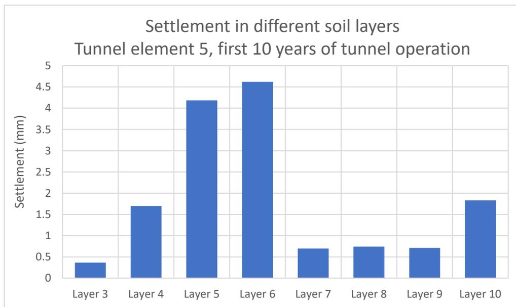
**Figure 7.8:** The histogram of soil settlement throughout the operational period
