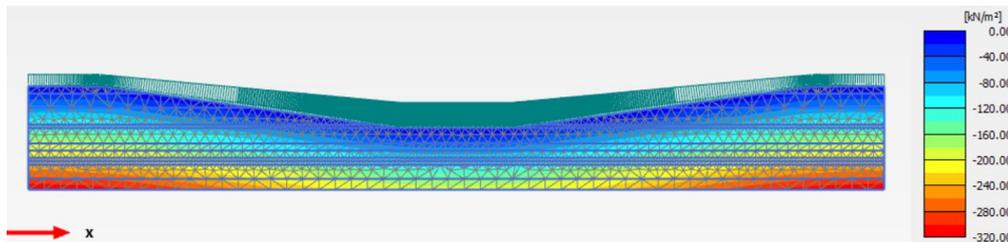
**Figure 4.8:** The effective stress of soil under trench excavation
