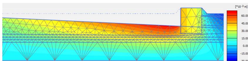
**Figure 6.5:** Settlement due to the excavation of approaching ramps
