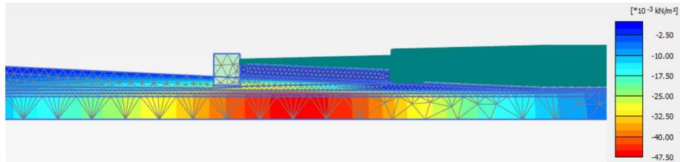
**Figure 6.16:** Excess pore pressure (0.047kPa) due to installation of tunnel element 1
