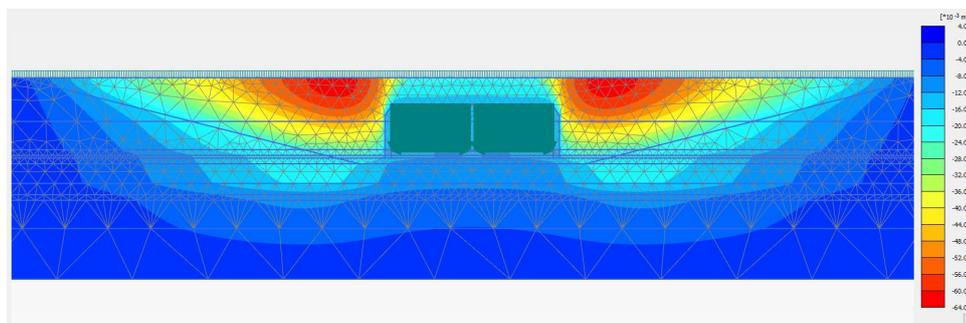
**Figure 4.12:** Settlement on sand backfill
