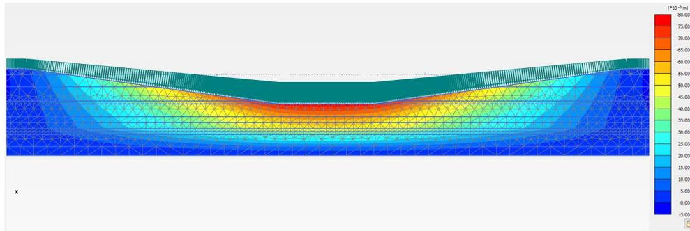
**Figure 4.7:** The unbonding result in the Plaxis model
