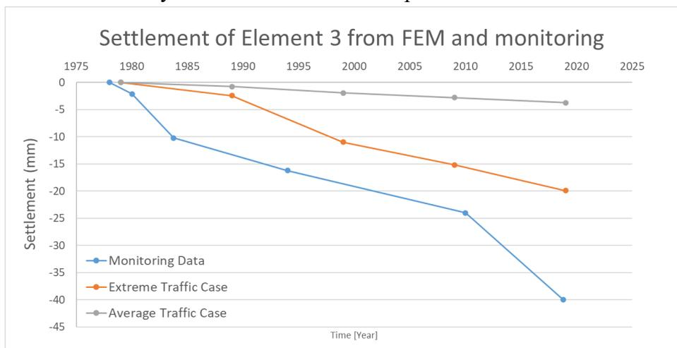
**Figure 4.23:** Settlement result comparison in Element 3
