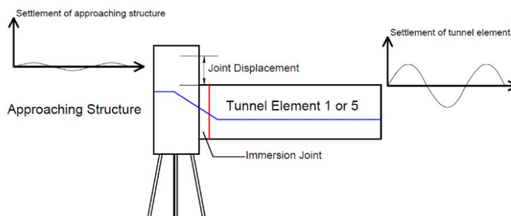
Figure 5.19: Joint displacement between approaching structure and tunnel element
