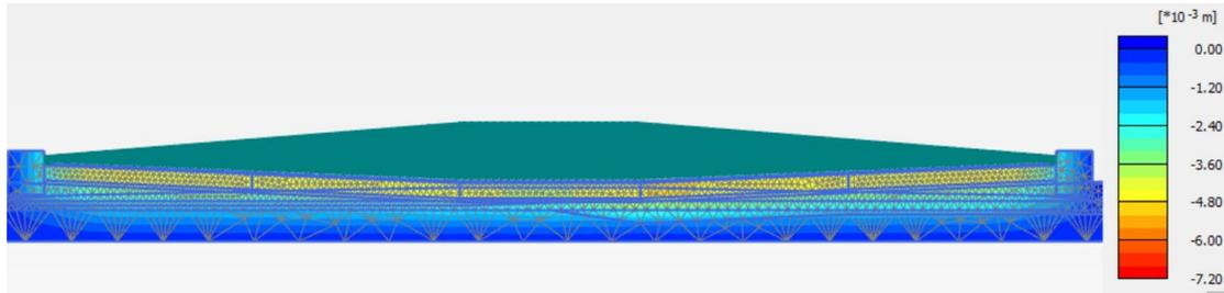
**Figure 6.21:** The settlement of immersed tunnel due to sand backfill
