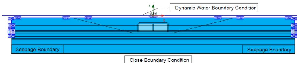
**Figure 5.5:** The hydraulic boundary condition of the soil domain
