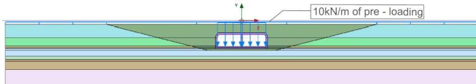
Figure 5.3: The pre-loading stage of soil domain
