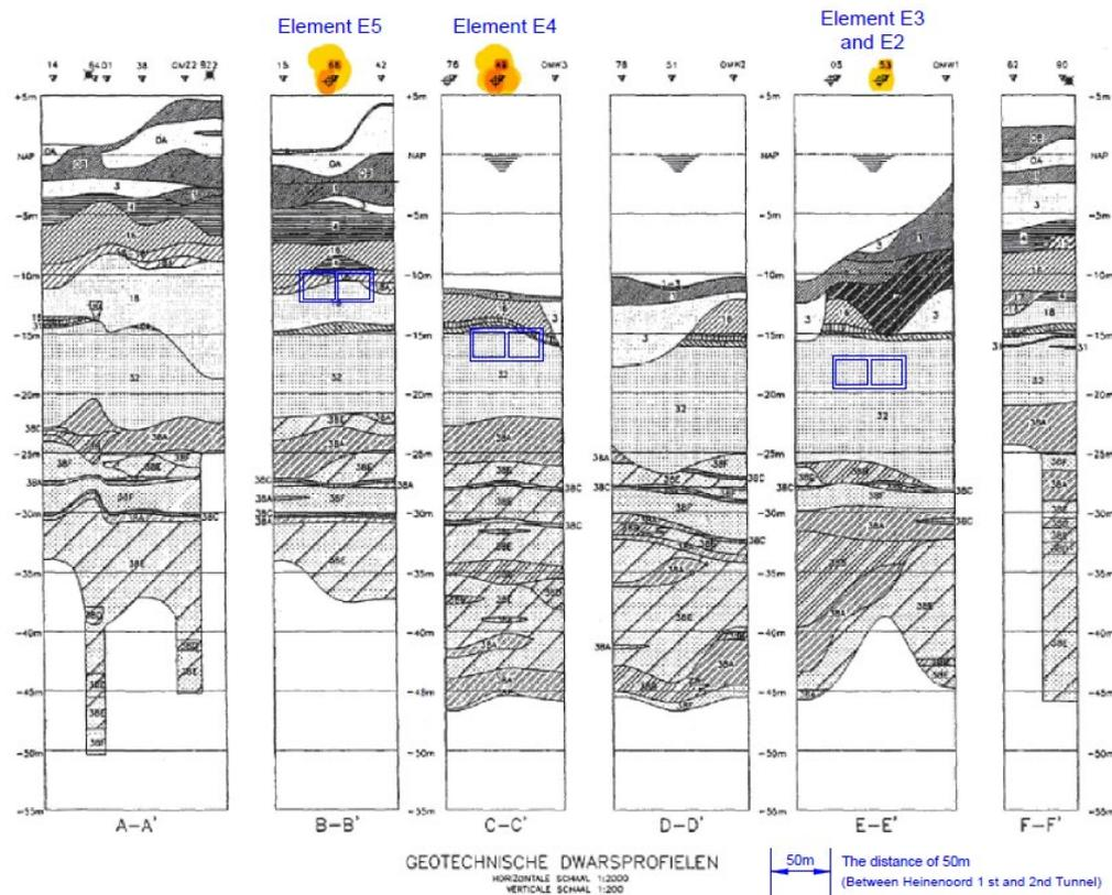
**Figure 3.3:** The location of bored hole and traverse tunnel section
