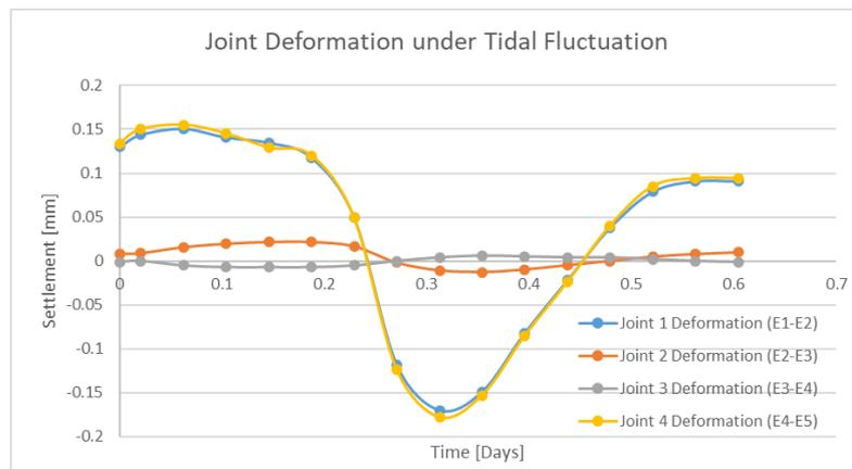
**Figure 6.36:** Joint deformation between tunnel element under tidal fluctuation
