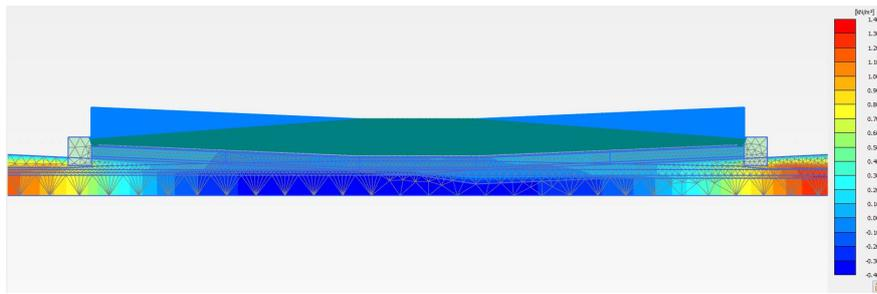
**Figure 6.30:** Excess pore water pressure of Heinenoord tunnel under tide
