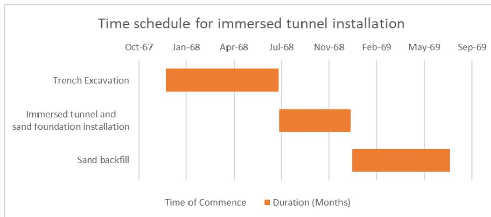
**Figure 4.6:** The time schedule of the immersed tunnel construction
