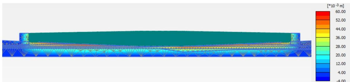
**Figure 6.7:** Settlement of soil rebound due to trench excavation
