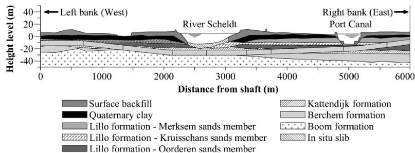
Figure 2.7: The longitudinal profile of Liefkenshoek tunnel under different geological unit
