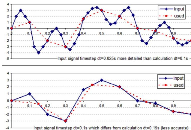
Figure 5.21: The difference between dynamic steps and input signal in Plaxis
