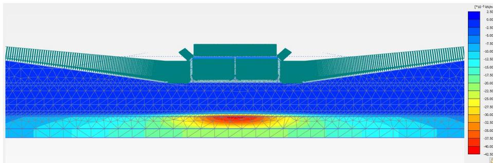
**Figure 4.11:** Excess pore water pressure under tunnel construction
