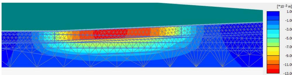
**Figure 6.15:** Settlement (1.122 cm) due to the installation of tunnel element 4
