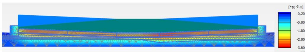
Figure 6.26: Settlement of Heinenoord tunnel under loading of 10kN/m
