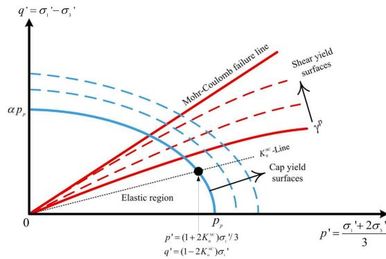
Figure 4.2: Double hardening yield contour of HS model
