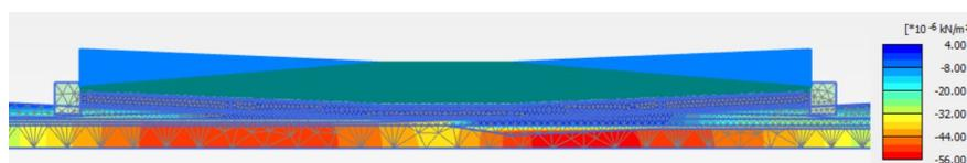
Figure 6.28: The excess pore water pressure of soil domain in phase 11
