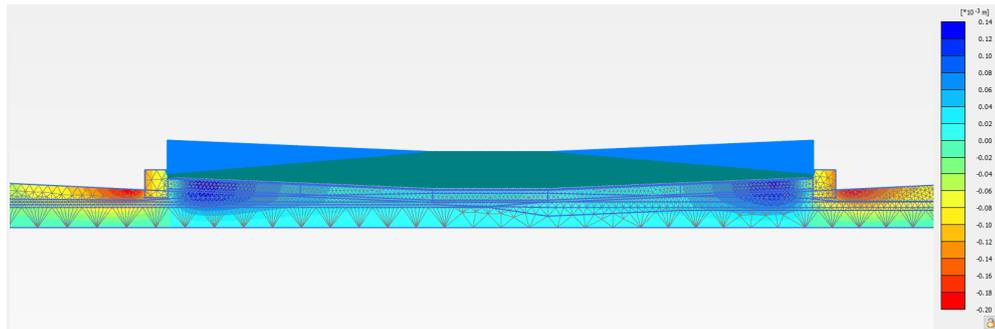
**Figure 6.33:** Settlement of immersed tunnel under the trough of the tide
