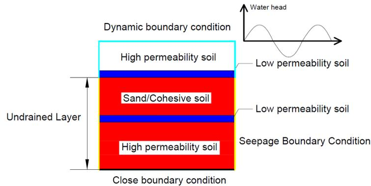
Figure 7.5: The hydraulic behavior of soil under the tidal variation
