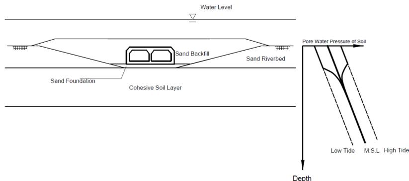
**Figure 5.4:** The pore water pressure along the soil domain under tide
