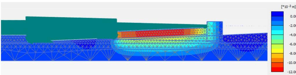
**Figure 6.14:** Settlement (1.172 cm) due to the installation of tunnel element 5
