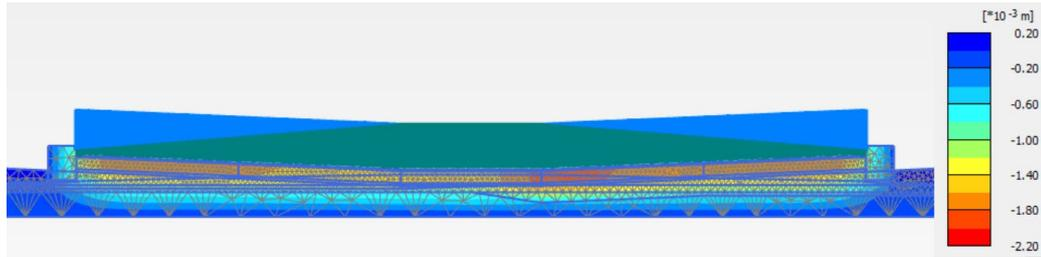
**Figure 6.23:** Settlement of Heinenoord tunnel after 10 years of operation
