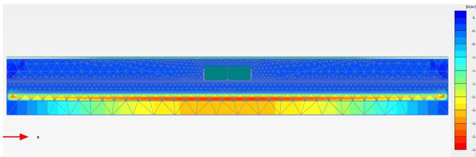
**Figure 5.13:** Excess pore water pressure of foundation soil under high tide
