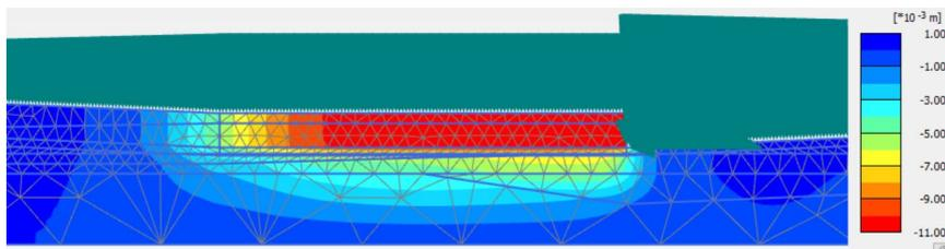
**Figure 6.13:** Settlement (1.101 cm) due to the installation of tunnel element 3
