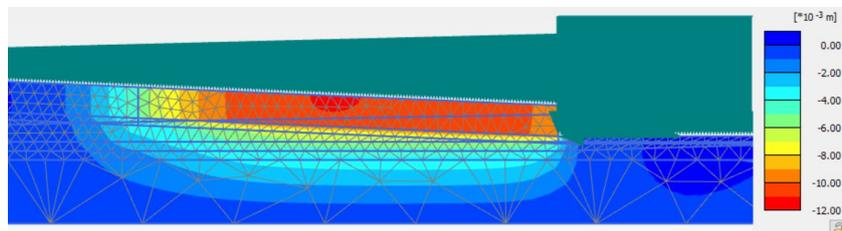
**Figure 6.12:** Settlement (1.102 cm) due to the installation of tunnel element 2
