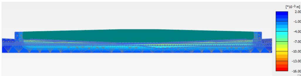
**Figure 6.9:** Settlement due to sand foundation installation
