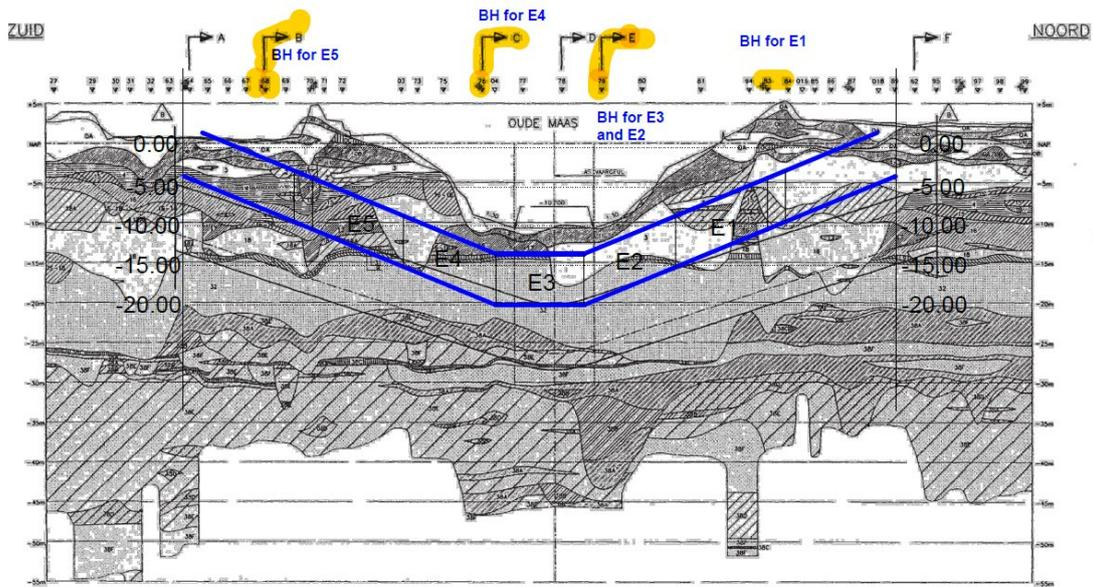
**Figure 3.2.** The longitudinal profile and bore hole location of Heinenoordtunnel
