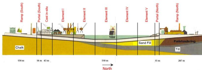
Figure 2.3: Geological profile of Limfjord Tunnel
