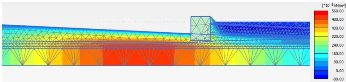
**Figure 6.6:** The distribution of excess pore water pressure under ramp construction
