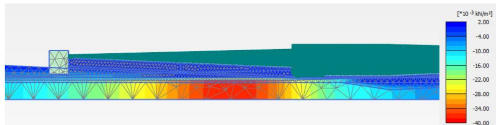
**Figure 6.17:** Excess pore pressure (0.038kPa) due to installation of tunnel element 2
