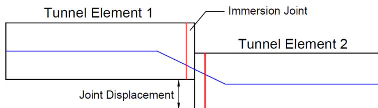
Figure 5.17: The differential settlement across tunnel element 1 and 2
