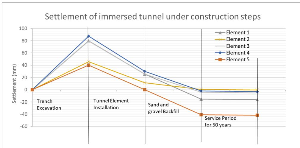
**Figure 4.15:** Settlement of immersed tunnel element under different time
