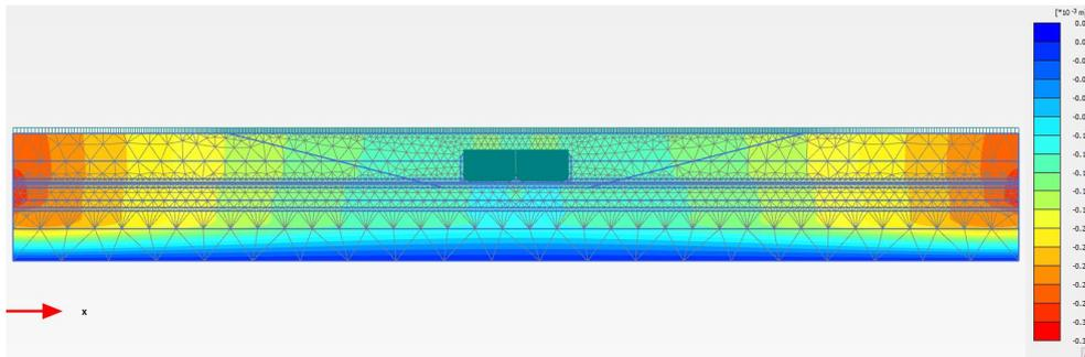
**Figure 5.12:** Settlement of immersed immersed tunnel under high tide
