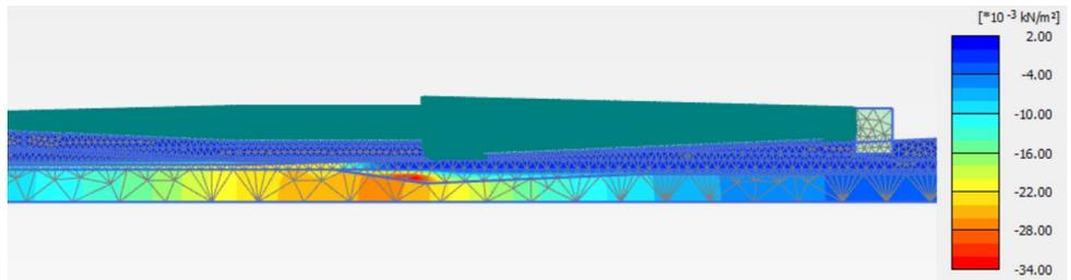
**Figure 6.18:** Excess pore pressure (0.033kPa) due to installation of tunnel element 3
