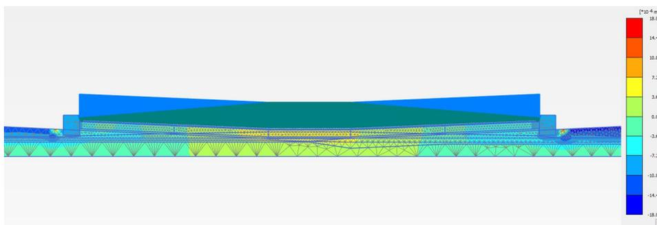
**Figure 6.31:** Settlement of immersed tunnel under mean water level
