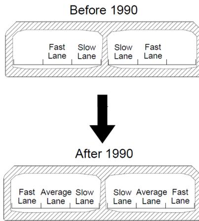
**Figure 4.19:** The change of traffic arrangement in Heinenoord tunnel
