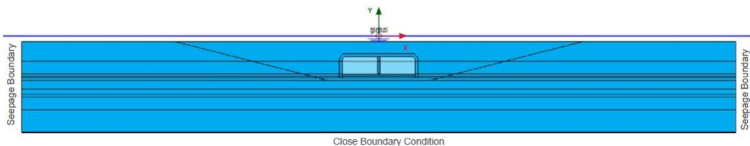
Figure 4.5: Hydraulic boundary conditions of tunnel element
