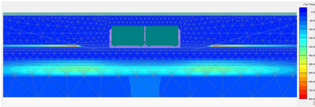
**Figure 4.13:** The excess pore water pressure during the sand backfill process
