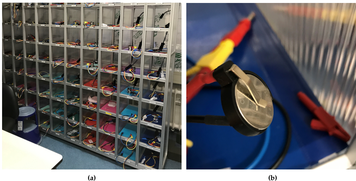
Figure 27: The coin cell cycling setup used during this research with (a) the battery cycling room and (b) a individual coin cell test setup.
