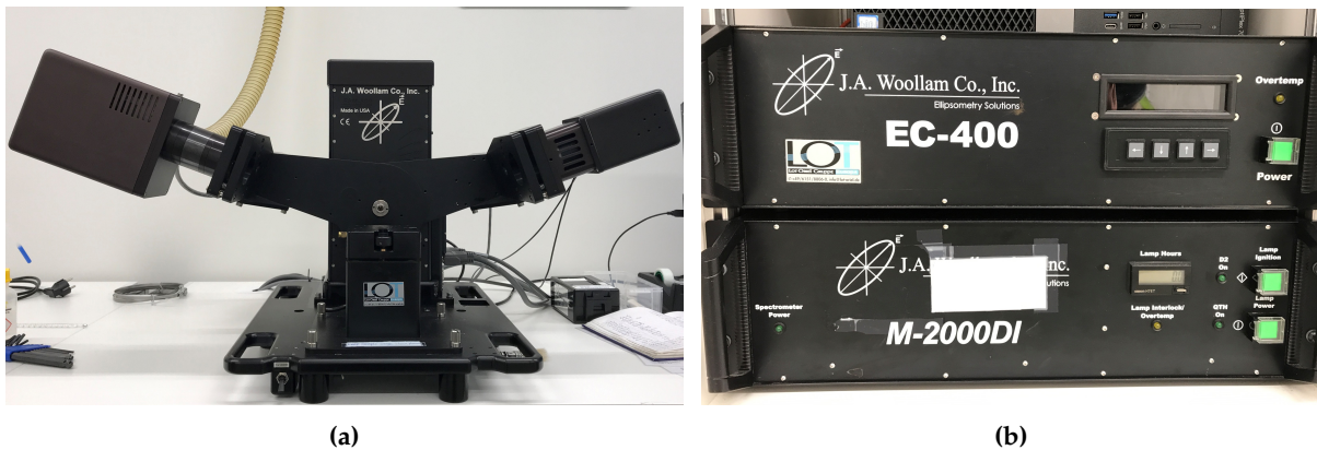
Figure 17: The spectroscopic ellipsometry machine used in this research to determine deposition rate, (a) the light source and polarizer head and the detector head with sample stage, (b) the J.A. Woollam power source.
