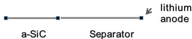
Figure 49: The 1D COMSOL battery model, consisting of a porous a\text{-SiC}_x\text{:H} cathode, a separator and a lithium metal anode [38].
