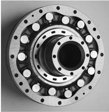
(a) View of the cam ring, pistons and rollers inside a Häggglunds Compact hydraulic motor (also applicable as pump) [11]
