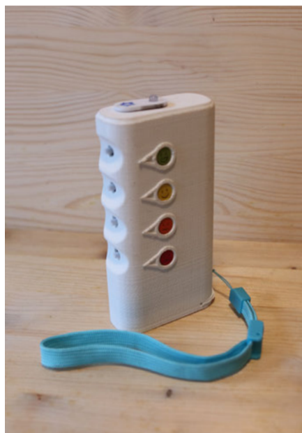
Figure 56. 3D print of the tracking device
