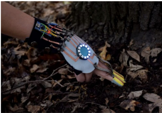
Figure 12. Hand-substrate interface (2018) by J Liu et al. : the wearer has to insert the finger into the soil to probe its moisture level, cultivating an embodied understanding of the relationship between fungal flourishing and soil condition. (Image credit: Jen Liu).
