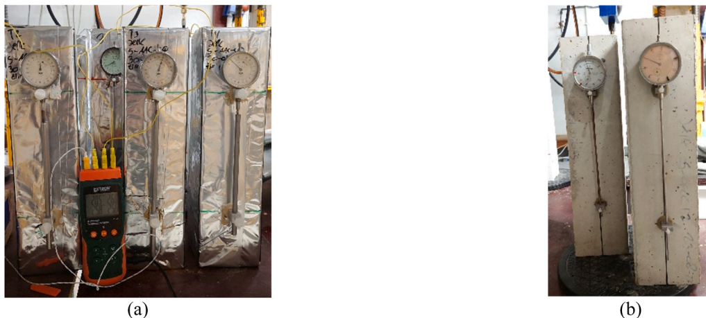
Fig. 1. (a) Sealed concrete prisms instrumented with a thermocouple and measurement clocks and (b) unsealed concrete prisms instrumented with measurement clocks.
