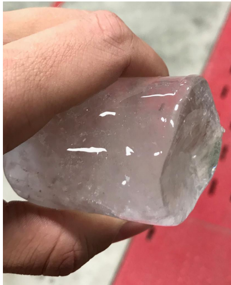
Figure C.5: Photograph of an ice puck after test where the ice and concrete were not well aligned and ice is partly molten away.
