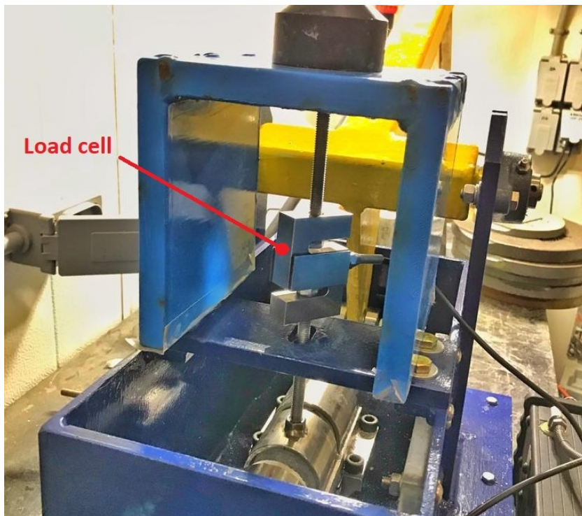
Figure D.1: Final set-up with extra load cell attached
