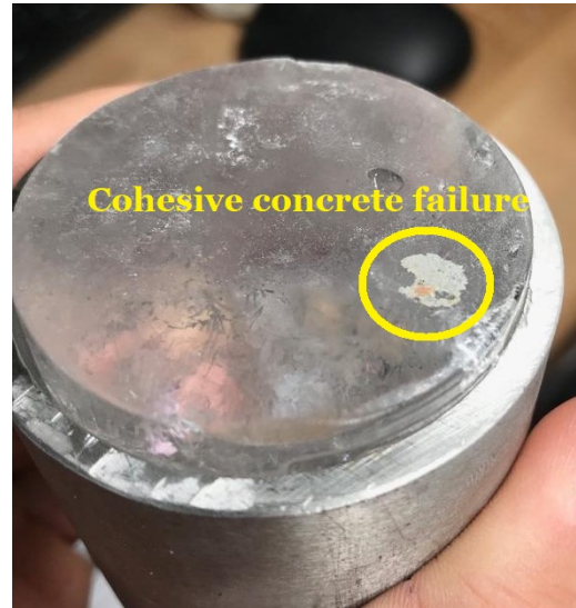
(b) Photograph of an ice puck after 682 kPa, 5 minute hold time test showing substrate failure of the concrete
