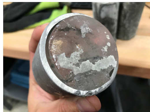
(b) Photograph showing ice surface after 682 kPa 20 min hold time test, where a thin layer of concrete paste can be seen stuck on the ice
