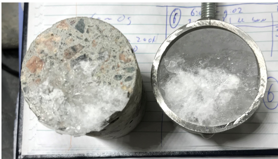
(c) much damage to the ice, going into the ice puck holder after 682 kPa pressure overnight test
