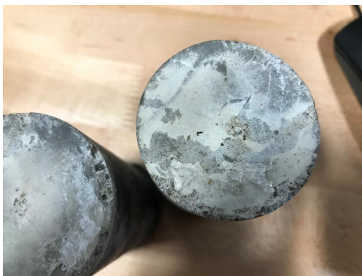
(a) Photograph showing paste surface after 682 kPa 20 min hold time test, where substrate failure of the concrete has been observed
