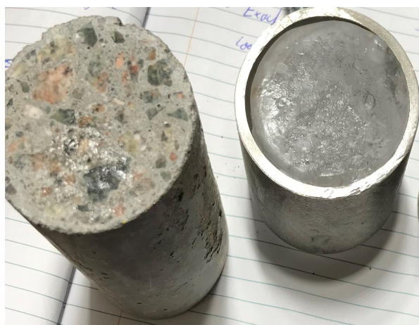
Figure C.4: Ice and concrete after shearing from 5 minutes 682 kPa test
