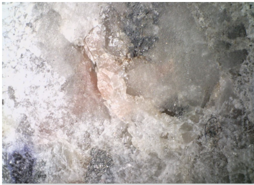
(c) Microscope image of concrete (a) after substrate failure of 682 kPa pressure and 5 minute hold time test
