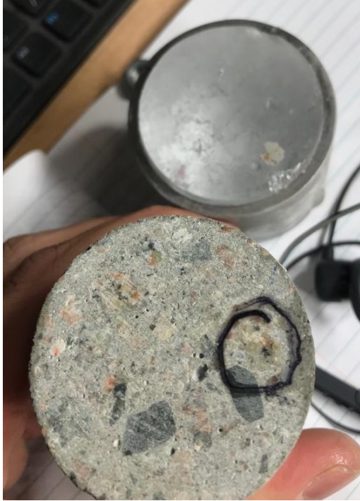
(a) Photograph of an ice puck and concrete cylinder after 682 kPa, 5 minute hold time test showing substrate failure of the concrete
