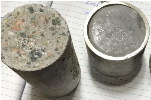
(a) Little portion of ice stuck on concrete after shearing, 682kPa and 5 minute hold time
