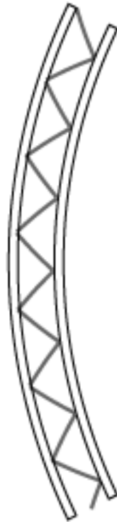
Buckling of a sandwich panel. Own image.
