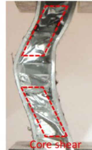
Failure modes aluminium sandwich panels with honeycomb core. Image by sun, Huo, Chen & Li, 2017.
