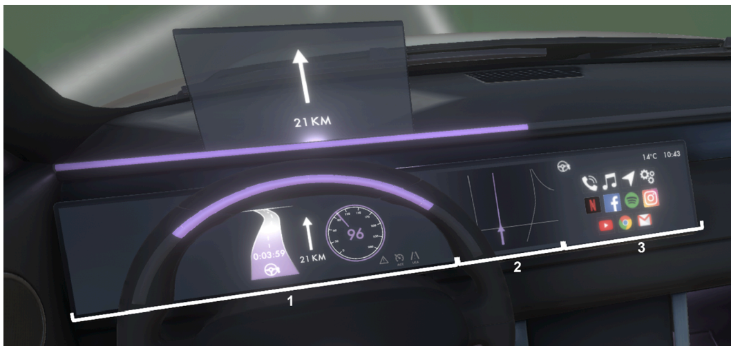
Fig. 2. The three sections on the long rectangular display (from left to right: (1) in front of driver, (2) next to steering wheel and, (3) in line with the center console) of the HMI’s display and the head-up-display (HUD) in ‘Stand-By’ (SB), as designed in Phase 2.
