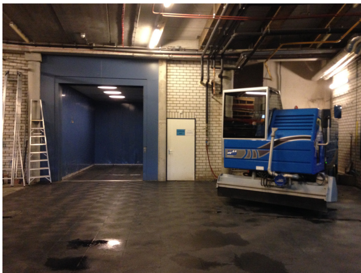
Parking place of the ice resurfer, behind the vehicle is a well to drop the scraped snow in from the ice (own picture).
