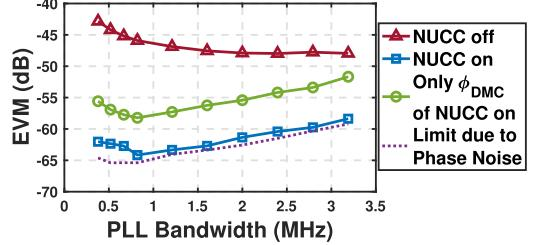
Fig. 12. Simulated EVM versus PLL bandwidth under different NUCC settings. The simulation conditions (i.e., PM signal, reference frequency  $f_{REF}$ , carrier frequency  $f_0$ , feedforward division ratio  $K$ , and so on) are the same as those in Fig. 20(b).
