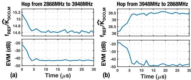
Fig. 25. Measured transient trajectories of the calibration coefficients and EVM. Modulation and calibration are turned on at  $t = 0$  after PLL gets locked to the target frequency  $f_0$ . Results are measured at  $K = 4$ , when  $f_0$  hops (a) from 2868 to 3948 MHz and (b) vice versa.
