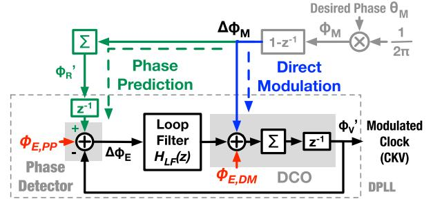
Fig. 2. Discrete-time domain model of an ideal PLL-based phase modulator with a two-point modulation. The gains of DCO and phase detector, respectively,  $K_{\text{DCO}}$  and  $K_{\text{PD}}$ , are implied as normalized, as in [27], hence hidden.
