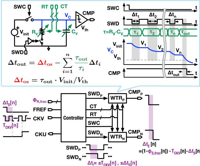
Fig. 16. Simplified diagram and waveforms of the TAU, which utilizes differential WTRs to calculate the weighted sum of input times (i.e.,  $T_{CKV}$  and  $\Delta t_S$ ) and outputs the result as  $\Delta t_E$ .
