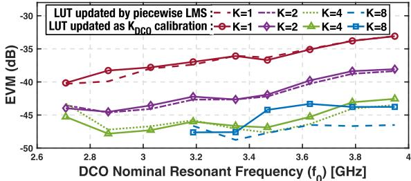
Fig. 24. Measured EVM versus the DCO carrier frequency ( $f_0$ ) at different forward frequency division ratios ( $K$ ). The corresponding  $BW_{FM}$  scales with  $K$ , i.e.,  $BW_{FM} = K \times 24$  MHz.
