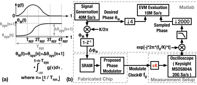
Fig. 19. (a) M-PSK signal generation by interpolating the symbol phases ( $\theta_{sys}$ ) with a frequency pulse-shaping filter [ $g(t)$ ] and (b) setup for measuring the phase modulator's EVM.
