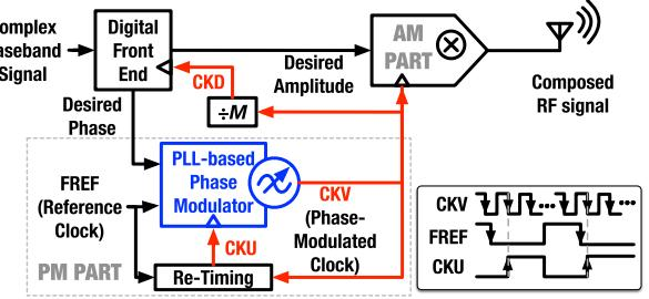
Fig. 1. Block diagram of a digital polar TX. The DCO-update clock, CKU, is obtained by re-sampling and inverting the reference clock, FREF, by the falling edges of the DCO variable clock, CKV.
