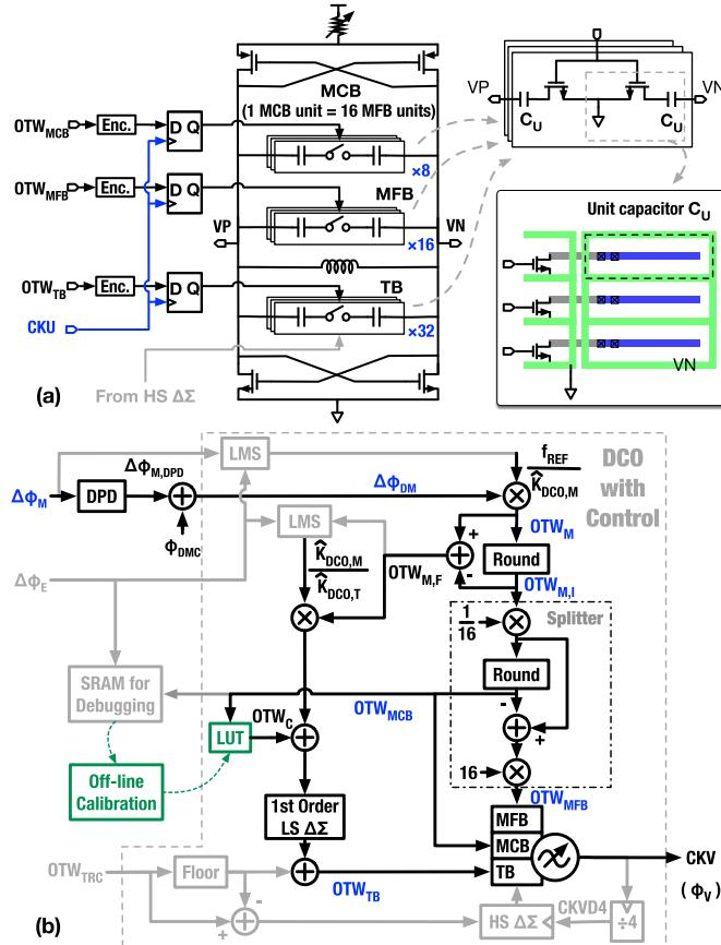
Fig. 13. (a) Schematic of the DCO core and (b) control logic surrounding the DCO core, where the digital blocks are implicitly clocked by CKU, except for the CKV clock divider ( $\div 4$ ) and the high speed (HS)  $\Delta\Sigma$ .
