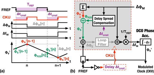
Fig. 4. Phase modulator with delay spread compensation: (a) waveforms and (b) block diagram.
