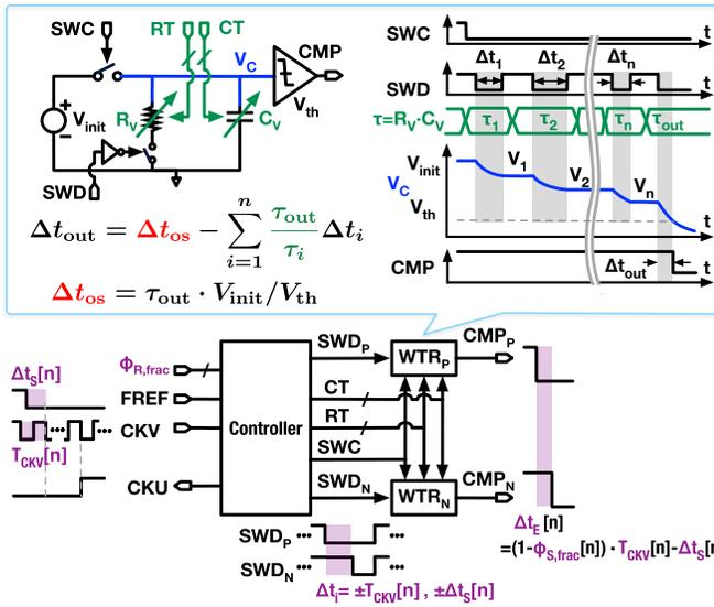
Fig. 16. Simplified diagram and waveforms of the TAU, which utilizes differential WTRs to calculate the weighted sum of input times (i.e.,  $T_{CKV}$  and  $\Delta t_s$ ) and outputs the result as  $\Delta t_E$ .
