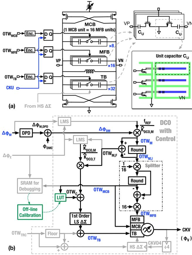
Fig. 13. (a) Schematic of the DCO core and (b) control logic surrounding the DCO core, where the digital blocks are implicitly clocked by CKU, except for the CKV clock divider ( $\div 4$ ) and the high speed (HS)  $\Delta\Sigma$ .
