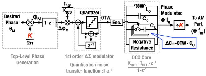
Fig. 9. Extracted open-loop representation in the direct-modulation path of the phase modulator, highlighting the influences of the forward frequency division ( $\div K$ ),  $\Sigma\Delta$  dithering and LC-tuning of the DCO.
