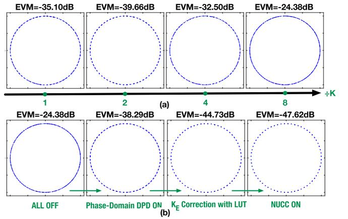
Fig. 20. Constellation diagram of a 60 Mb/s 64-PSK signal measured at  $f_0 = 3188$  MHz: (a) Feedforward frequency division  $K$  increases from 1 to 8, with all compensation options off (i.e., phase-domain DPD, LUT for OTW<sub>MCB</sub>, and NUCC) and (b)  $K = 8$  and all the compensation options are incrementally turned on.
