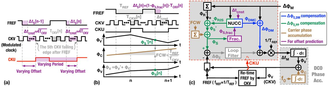
Fig. 5. Phase modulator with the proposed non-uniform clock compensation (NUCC): (a) Waveforms showing CKU generation by re-timing FREF by CKV, (b) waveforms illustrating the phases related to  $\Delta t_S$  prediction, and (c) system diagram.
