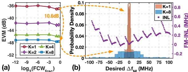
Fig. 23. (a) Measured EVM versus fractional FCW ( $\text{FCW}_{\text{frac}}$ ) for different feedforward frequency-division ratios ( $K$ ) when the integer FCW is fixed at 79 (i.e.,  $f_0$  around 3160 MHz) and (b)  $\Delta f_M$  distribution correlated with the DCO's FM-INL.
