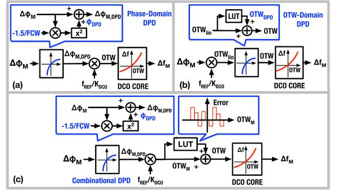
Fig. 10. Predistorting of DCO nonlinearity in (a) phase domain, (b) OTW domain, and (c) both domains, i.e., the combinational DPD.
