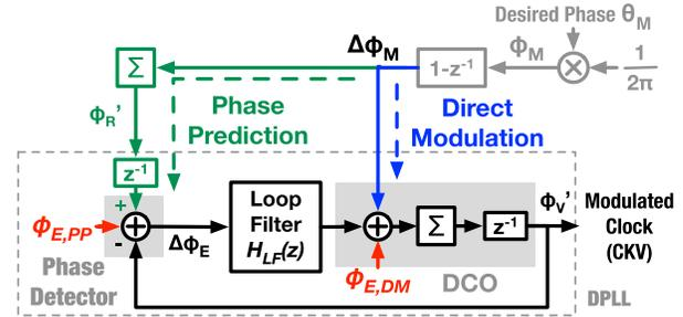
Fig. 2. Discrete-time domain model of an ideal PLL-based phase modulator with a two-point modulation. The gains of DCO and phase detector, respectively,  $K_{DCO}$  and  $K_{PD}$ , are implied as normalized, as in [27], hence hidden.
