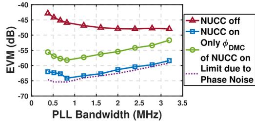
Fig. 12. Simulated EVM versus PLL bandwidth under different NUCC settings. The simulation conditions (i.e., PM signal, reference frequency  $f_{REF}$ , carrier frequency  $f_0$ , feedforward division ratio  $K$ , and so on) are the same as those in Fig. 20(b).
