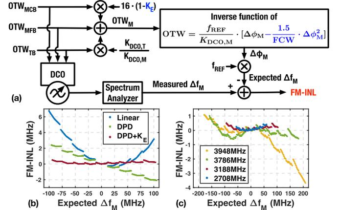
Fig. 18. DCO FM-INL: (a) Measurement setup, (b) measured results with different DCO linearization settings when  $f_0 = 3188$  MHz, and (c) measured results with the proposed phase-domain DPD and the same  $K_E = 0.023$  at multiple  $f_0$ 's.
