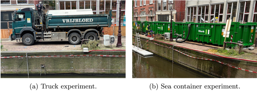
Fig. 4. Execution of the proof load test.
