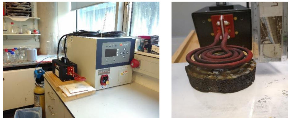
Figure 2. Ambrell Ekoheat 10 kW induction machine—laboratory induction apparatus.
