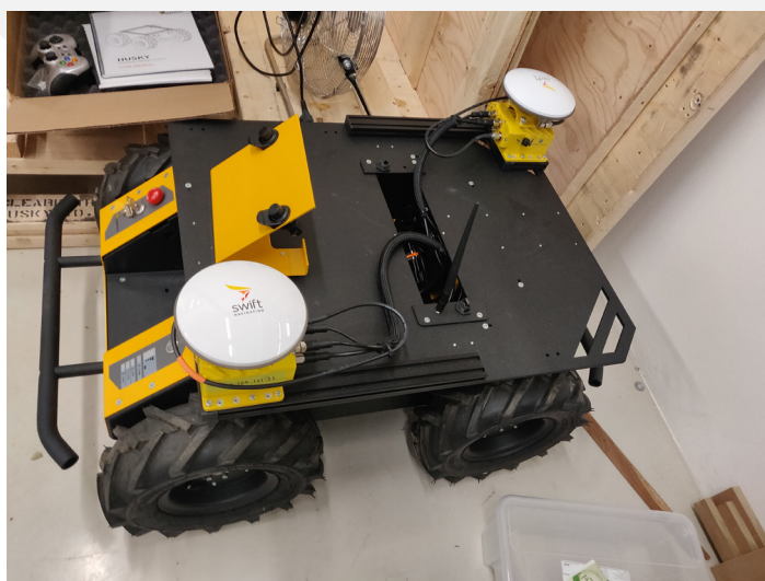
Figure 2.2.4. Husky with current sensors 9
