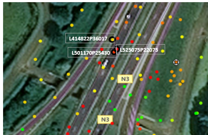
Figure D.2: SkyGeo points available and the three points used to extract data sets indicated for trajectory 1.1 of the N3
