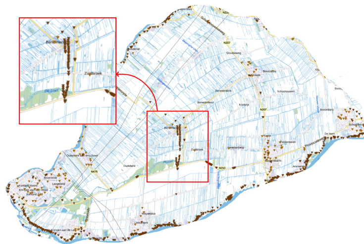
Figure B.2: Distribution of CPT profiles available in the Krimpenerwaard polder, CPT tests indicated with brown triangles. source: DINOloket
