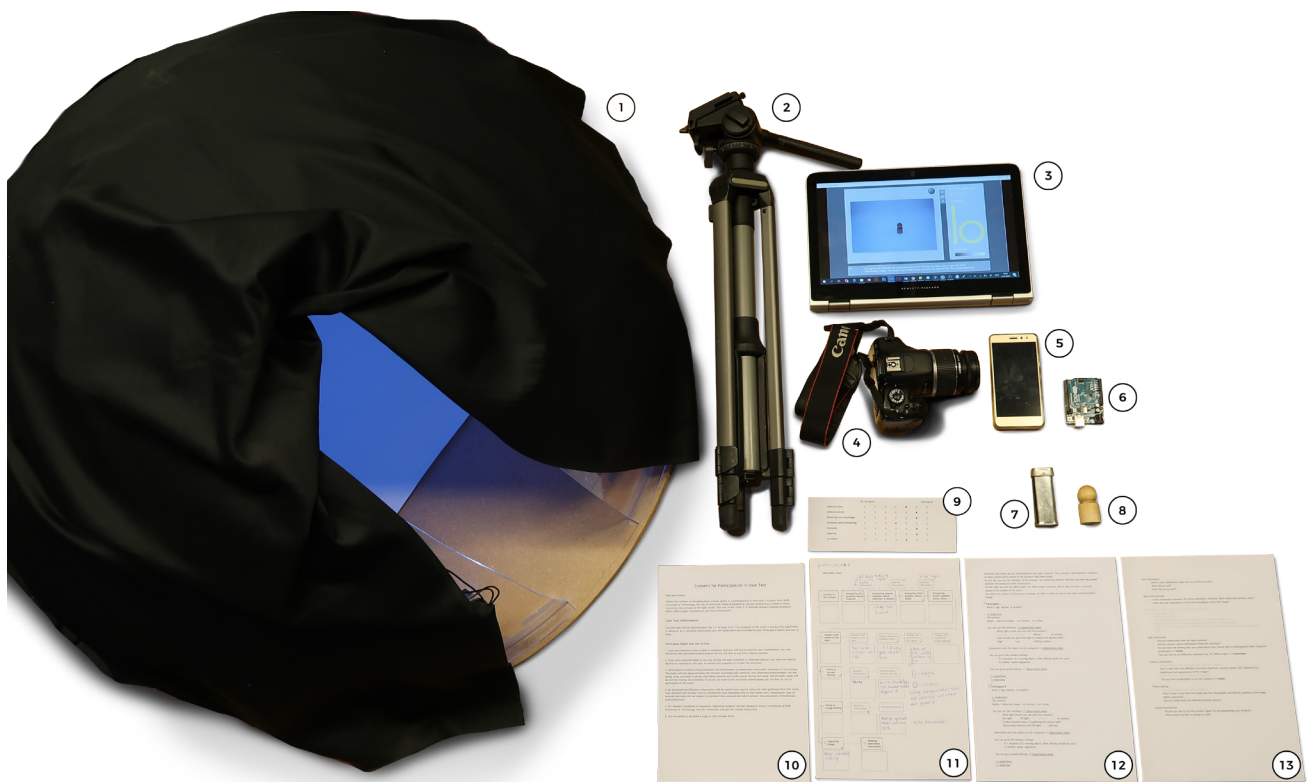
Figure 61, Stimuli used during the user test. (1) light studio, (2) tri-pot, (3) laptop with the interface, (4) DSLR camera with zoom lens, (5) phone for recordings, (6) Arduino UNO for communication from laptop to light studio, (7) first test object, (8) second test object, (9) Likert scale question form, (10) consent from allowing audio recording and rights for the participant, (11) observation sheet, (12) procedure per participant, and (13) interview questions.
