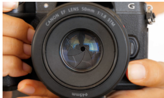
Figure 11, The aperture blades are placed behind the lens of the camera and determines how much light reaches the sensitive sensor (Feather & the wind, 2018)
