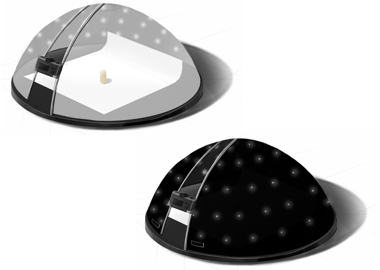
Figure 68, Final product. Lights on the outside will indicate where the light is located. A hinge will make it possible to easily place a subject inside. A softbox cap can be placed inside for diffuse light.
