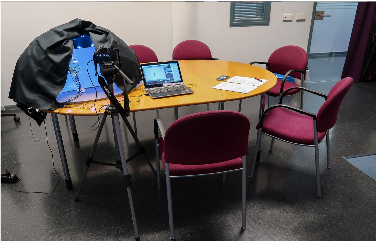
Figure 63. Test setup. The light studio is placed on the left with the camera in front. The laptop with interface is placed on the right. The participant was sitting on the left chair and the facilitator on the right chair.
