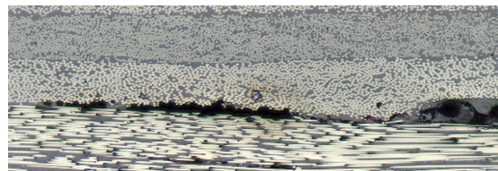
(b) Heat induced delamination
