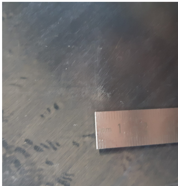
Figure C1: Fiber damage on the non-impacted side of specimen 1.2
