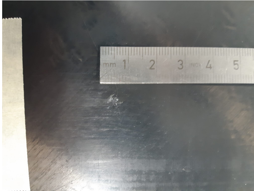
Figure C2: Fiber damage on the non-impacted side of specimen 1.9
