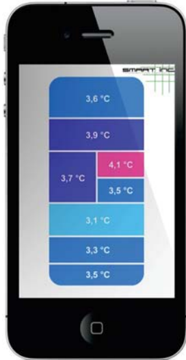
Figure E11. Smart refrigerator and a mobile application that supports the reduction of energy use by adjusting to peaks in energy network. Designers: Bram van Wijk and Robbert Bakker.
