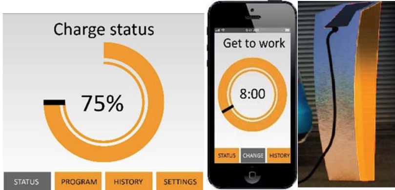
Figure E22. Electric vehicle power station with user interface that supports smart charging of electric vehicles and peak reduction in electricity use. Designers: Mattijs Stam and Abel Gerrits
