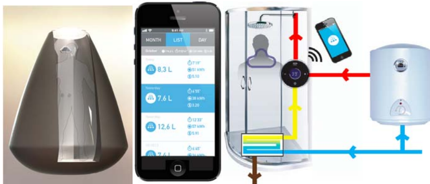
Figure E2. Innovative shower with digital application that supports the use of less hot water and energy.
