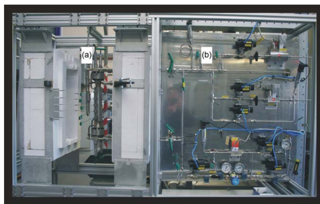
FIG. 3. (Color online) Schematic representation of the complete reactor setup. The left side (a) shows the reactor part and insulation, the right part (b) shows the gas handling system.
