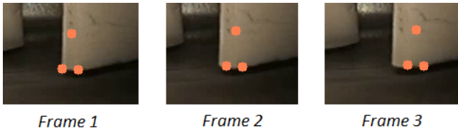
Figure 6: Lucas-Kanade on three consecutive frames of Video 1. The features are not tracked properly. Better results can be obtained with manual annotation. ( Experiment 2 )
