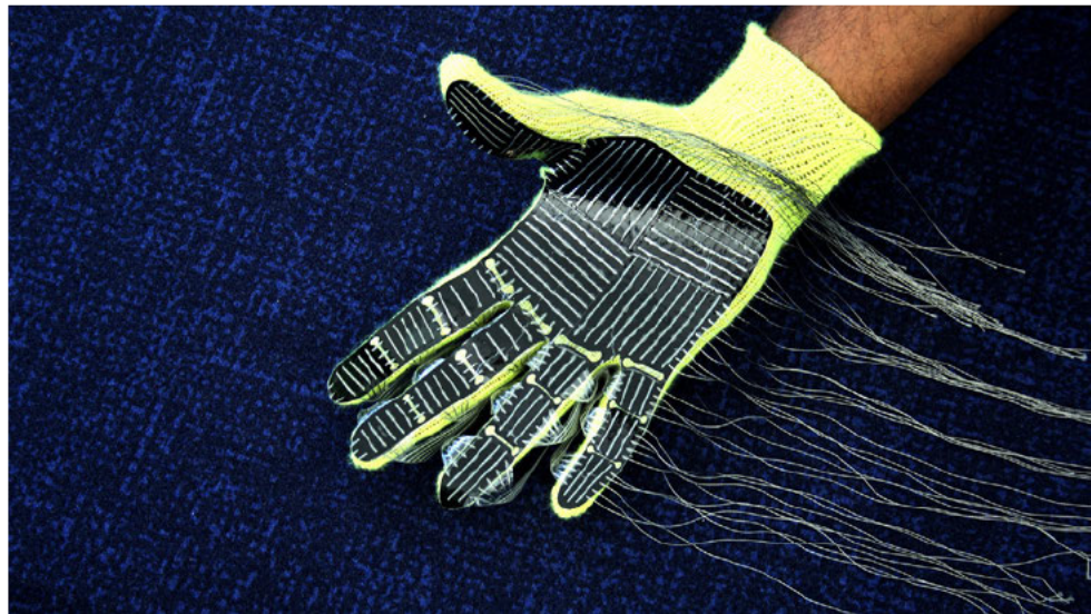
image / figure 1: MIT research on an electronic pressure sensing glove for human touch
