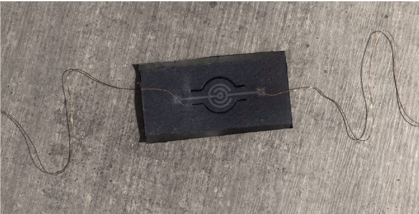
Figure 57 - embedded single sensor with visualisation overlay of internal structure
