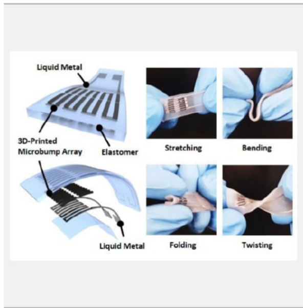
image / figure 2: 3DP technique of printing flexible pressure sensors
