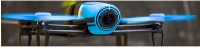
Fig. 6. A Parrot Bebop 1 is used as the flying platform. The original autopilot is fully replaced by an open-source autopilot called Paparazzi UAV.
