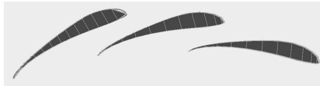
**Figure 3.3:** *Staggered wing design helps to direct the flow, which would have otherwise separated, according to the shape of the wings staggered behind the first wing. [own work]*
