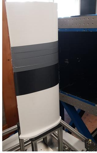
**Figure 5.1:** The 3D printed S1223 airfoil in front of the open jet wind tunnel.
