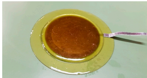
Figure 3. Dual layer epoxy sample with a 30 nm thickness gold electrode in-between layers.
