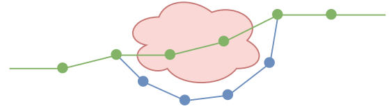
(a) Avoidance maneuver (blue path) around an obstacle (red cloud).
