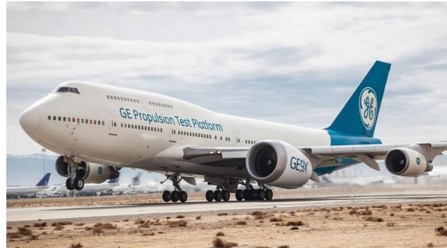
(b) General Electric GE9X Engine on a Boeing 747 Aircraft During an Engine Test Flight <sup>4</sup>
