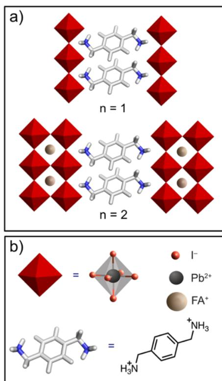
**Figure 1. Schematic representation of Dion-Jacobson layered hybrid perovskites.**
