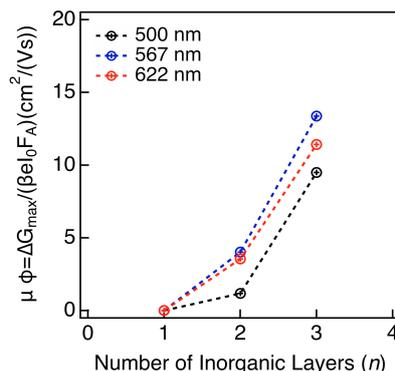
**Figure 5. Photoconductivity.** Maximum photoconductivity of thin films at 298 K based on  $(\text{PDMA})\text{FA}_{n-1}\text{Pb}_n\text{I}_{3n+1}$  composition ( $n = 1\text{--}3$ ) excited at the respective excitonic wavelengths (500 nm, 567 nm and 622 nm) of  $n = 1$  (black),  $n = 2$  (blue) and  $n = 3$  (red), respectively.
