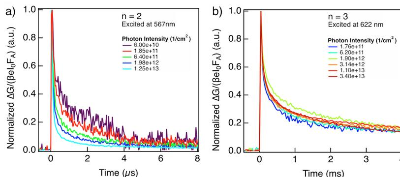
**Figure 6. Charge carrier dynamics.** Normalized photoconductivity as a function of photon intensity of (PDMA)FA<sub>n-1</sub>Pb<sub>n</sub>I<sub>3n+1</sub> thin films on quartz substrates based on (a)  $n = 2$  and (b)  $n = 3$  nominal compositions highlighting long lived-component in the order of  $\mu s$ –ms.
