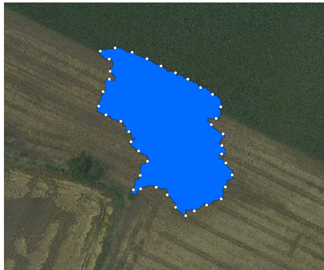
Figure 3.1: Overview of sampling the boundaries of the flooded polygon every 10 meters, over which the DEM values will be computed to extract the water levels.
