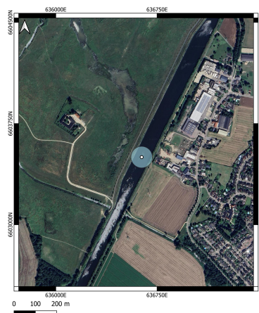
Figure 2.15: Example of the LMW gauge near Bunde, projected onto the center line of the river and the surrounding 50 meter radius that is assumed to have a constant water level.
