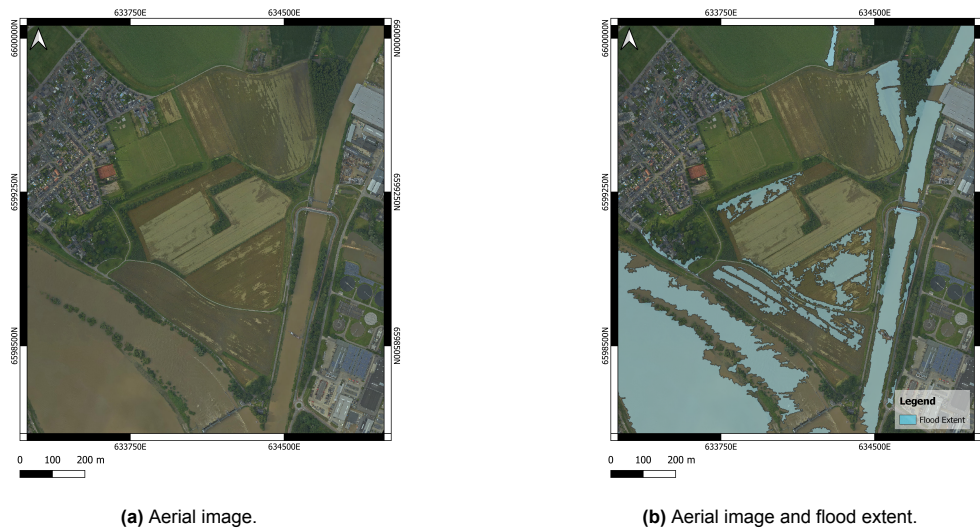
Figure 5.2: Example of puddle formation resulting in classification of flooded pixels.
