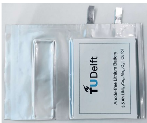
Fig. S6.44. Anode-free NCM811||Cu pouch cell. The anode-free NCM811||Cu pouch cell is after preparation.
