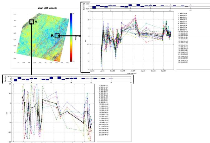
Fig.6. MLV of ground deformation in mm/year marked in Oulja (A) and Sahel (B) sectors.
