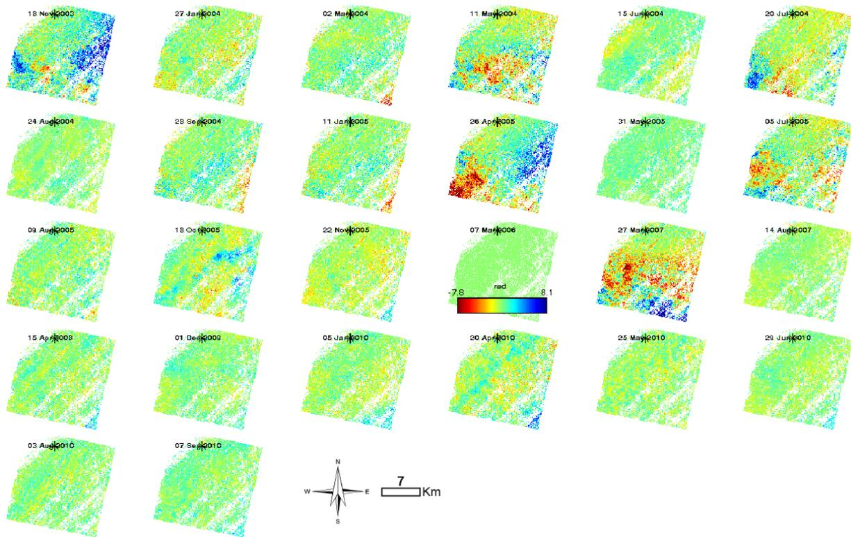
Fig. 4. The unwrapped phase of each interferogram referenced to the master image.
