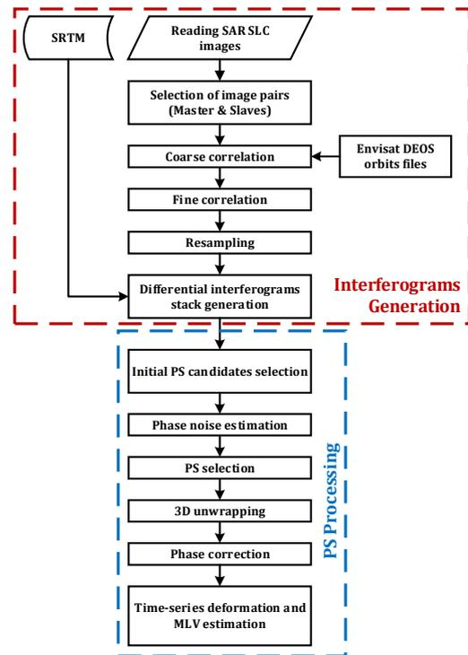
Fig.2. Framework used for estimating deformation.
