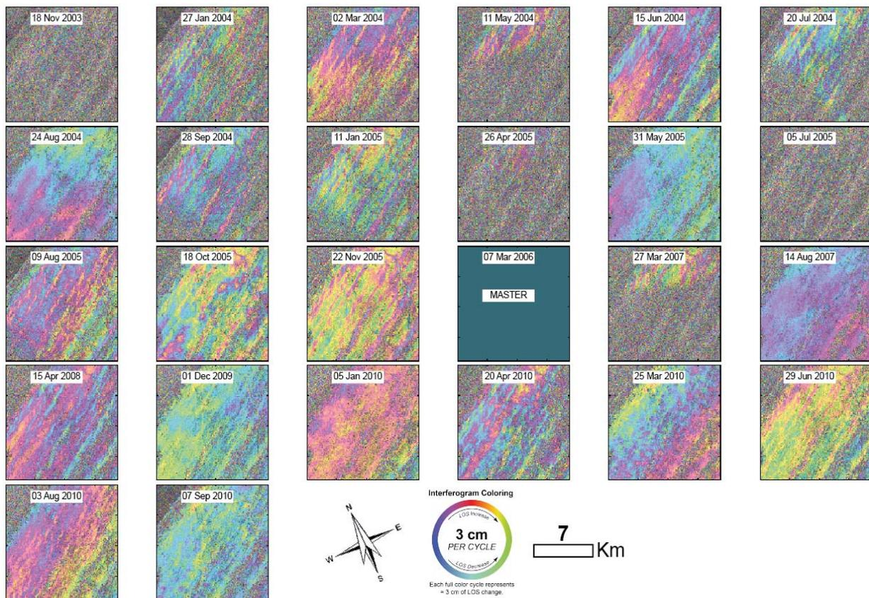
Fig. 3. Differential interferograms referenced to the master image (07-03-2006) after subtraction of reference phase and phase due to DEM (each full color cycle represents  $\approx 3$  cm of displacement in LOS direction).
