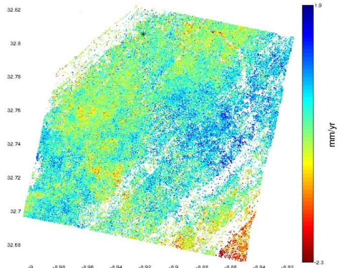
Fig. 5. Deformation expressed as Mean LOS Velocity (MLV) in mm/year relative w.r.t reference area (the asterisk mark in the North of the study area).
