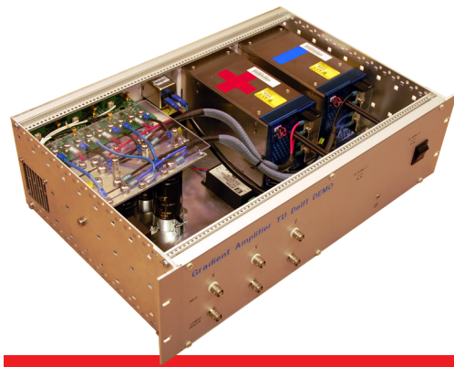
Figure 6. The new gradient amplifiers (x,y,z) built into a 19" subrack of 3U height.
