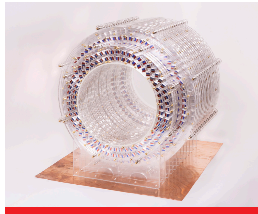
Figure 1. The current version of the low-field MRI. The picture shows the (permanent) magnet in which the patient's are inserted.
