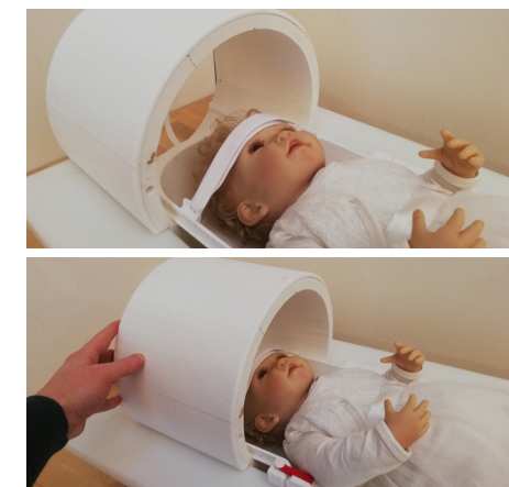
Figure 47. The crucial red strap, the placement of the patient, and the sliding of the coil over the patient's head.
