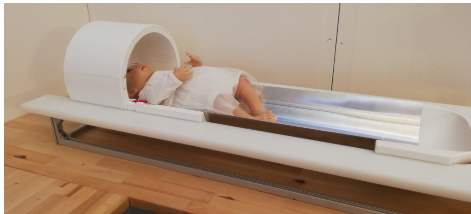
Figure 45. Prototype of the bed assembly, 1:1 scale.
