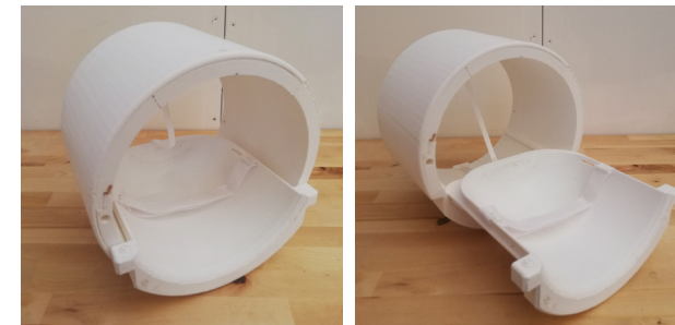
Figure 49. The coil and headrest. The straps work as intended, and do not get entangled or get in the way. The straps and attachments must be sufficiently strong to resist wear.
