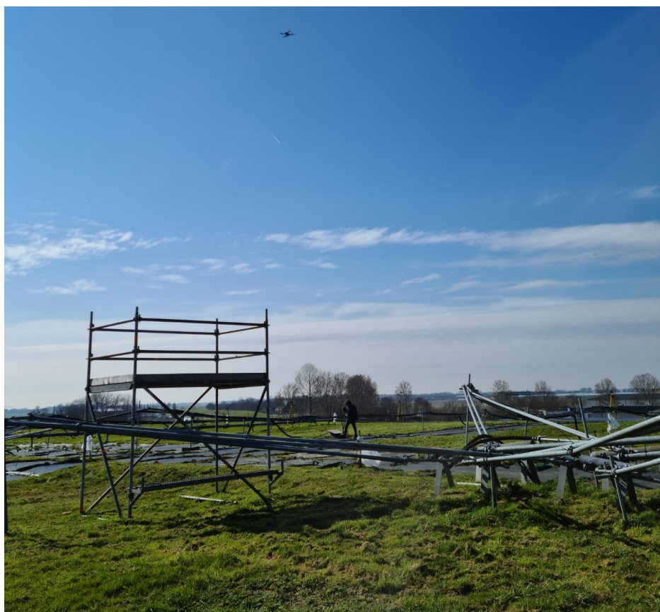
Figure A.8: Scaffolding and aeration infrastructure used for the registration of same-day ALS and TLS scans.
