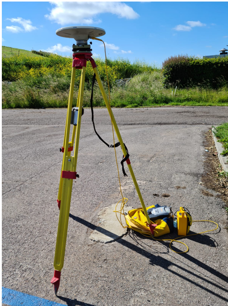
Figure A.4: Trimble R7 GNSS base installed on a nearby parking area.
