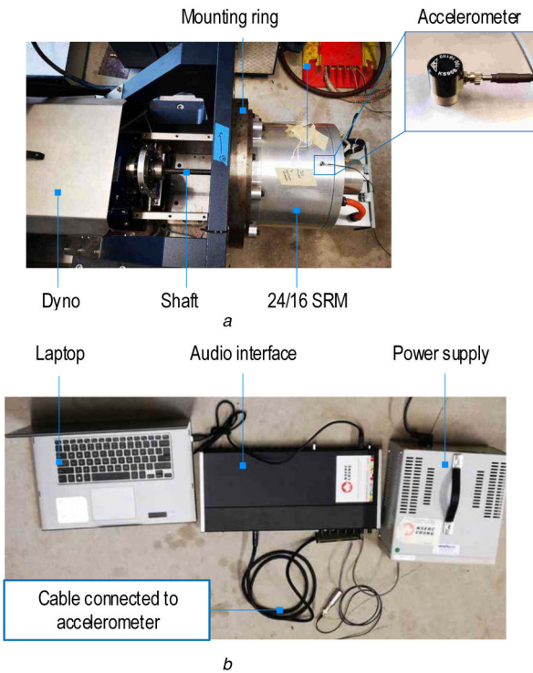
Fig. 21 Setup for the hammer test of the 24/16 SRM (a) 24/16 SRM mounted in the dyno, (b) Audio interface and power supply
