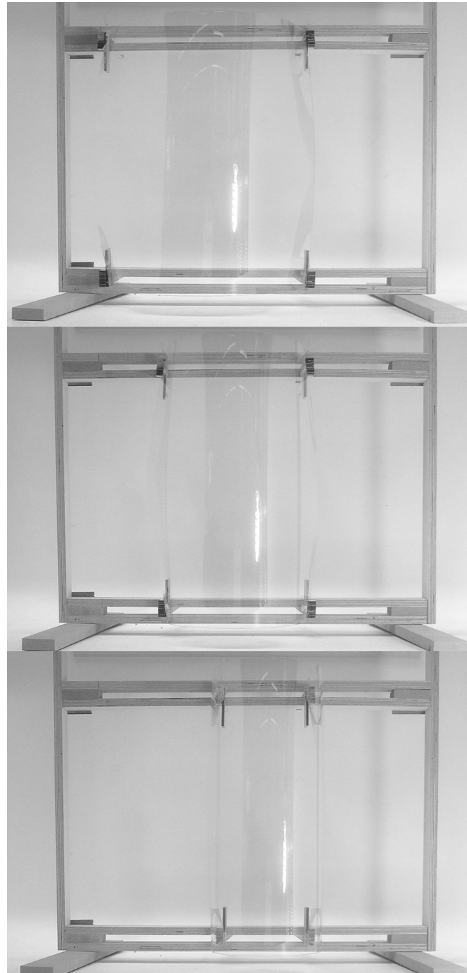
Figure 80-Increasing of bending of the physical model. Translation of the left edge.
