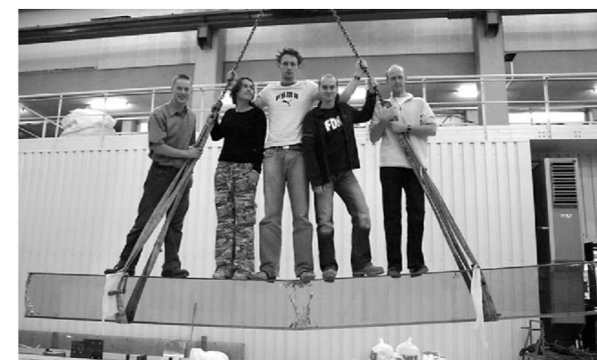
Figure 16-Laminated reinforced cracked beam supporting the weight of five people.
