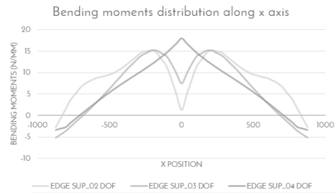
Chart 26-Bending moments distribution along x axis in the middle of the panel for edge supports configuration according to the number of degrees of freedom.
