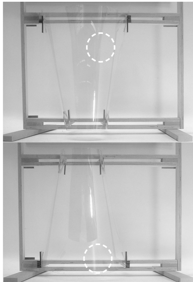
Figure 82-Asymmetric movement. Different radius on the top and bottom edge.
