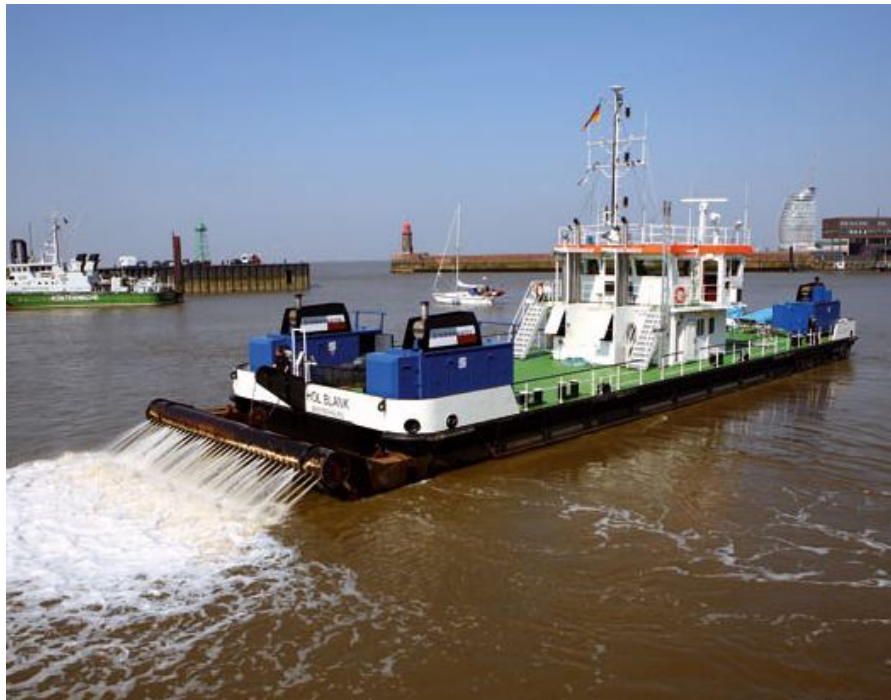
Figure 5.8: Example of a water injection dredge, the injection part will be lowered to the bottom (Dredging Today, 2014).
