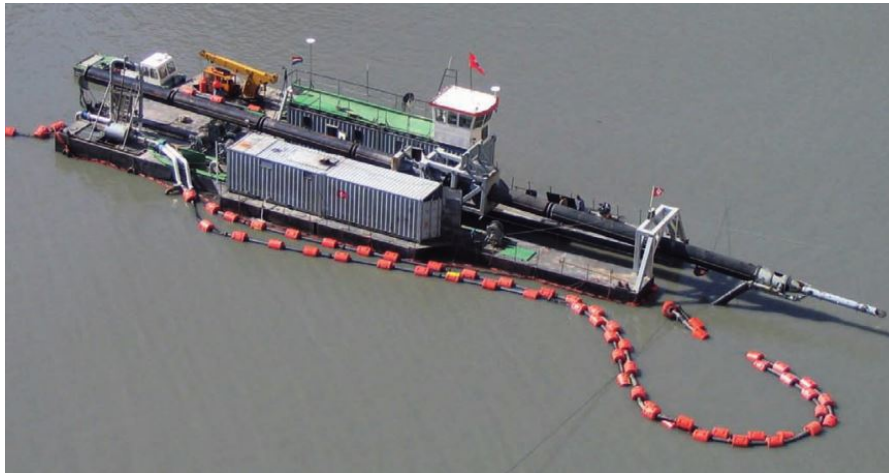
Figure 5.2: Example of a suction dredge (Baggerbedrijf de Boer B.V., 2014). Note the very long suction pipe used for reaching great depths.
