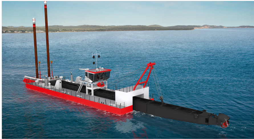
Figure 5.3: Example of a Cutter Suction Dredge (IHC, 2017).
