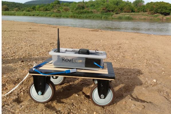
Figure B.2: Cart with the RTK GPS rover on top in order to measure the floodplain and exact waterline.
