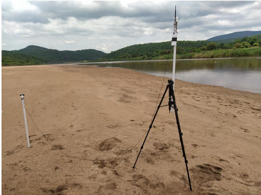
Figure A.2: Setup of the RTK base. Left the GNSS receiver and on the tripod the SimpleRTK2B board with radio module.
