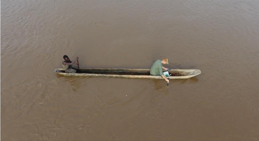
Figure A.4: Measuring the surface flow velocity with a current meter from a canoe.
