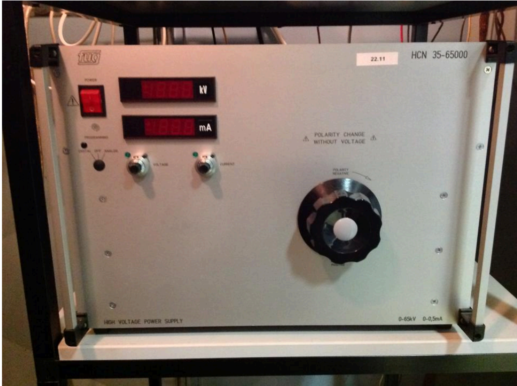
Figure 5.2.4: HVDC supply for PEA setup
