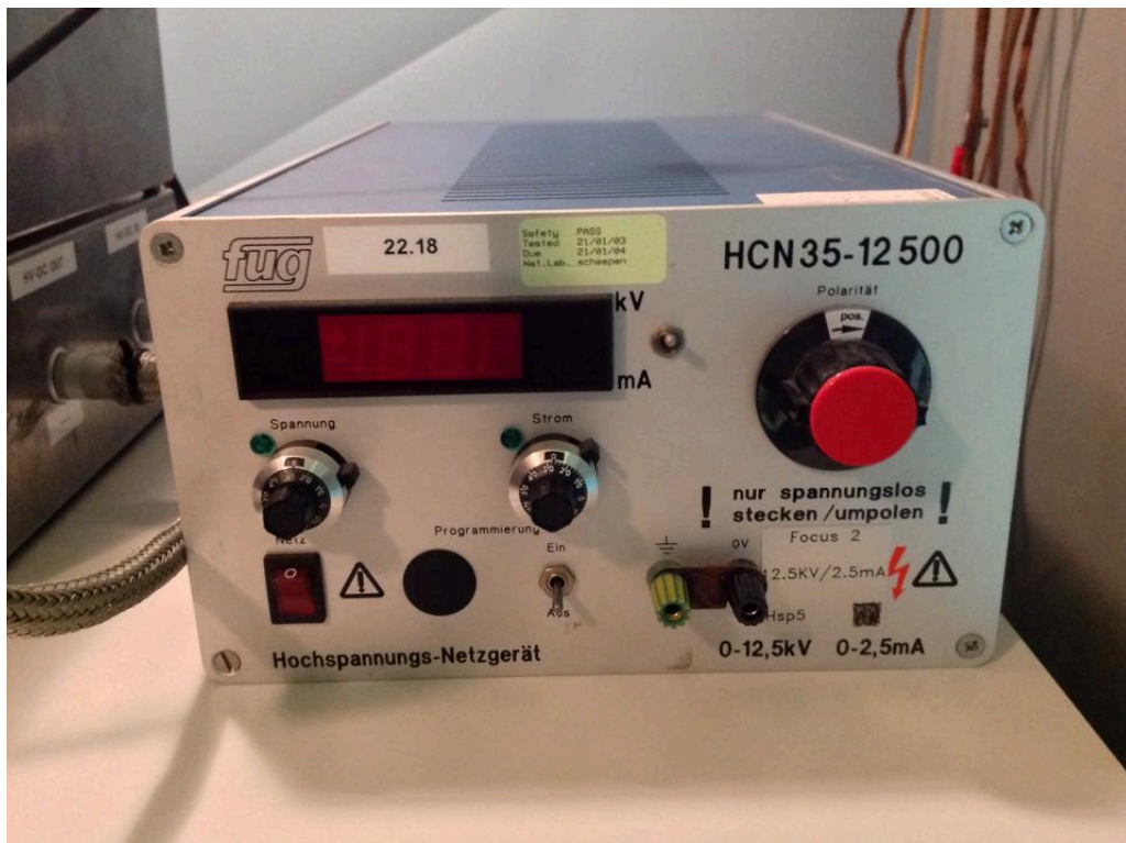
Figure 5.2.3: HVDC pulse generator for PEA setup
