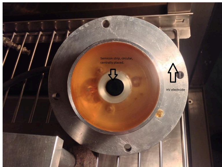
Figure 5.2.8: PEA setup, HV electrode with semicon strip
