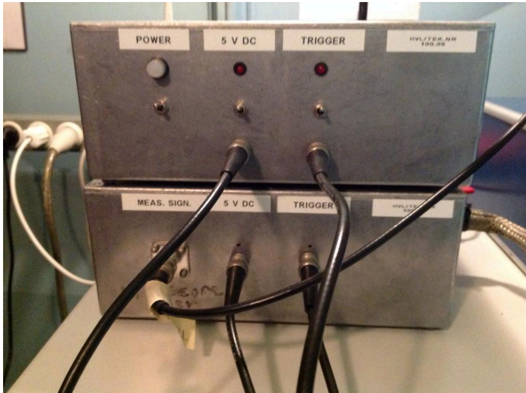
Figure 5.2.2: Switch box for PEA setup
