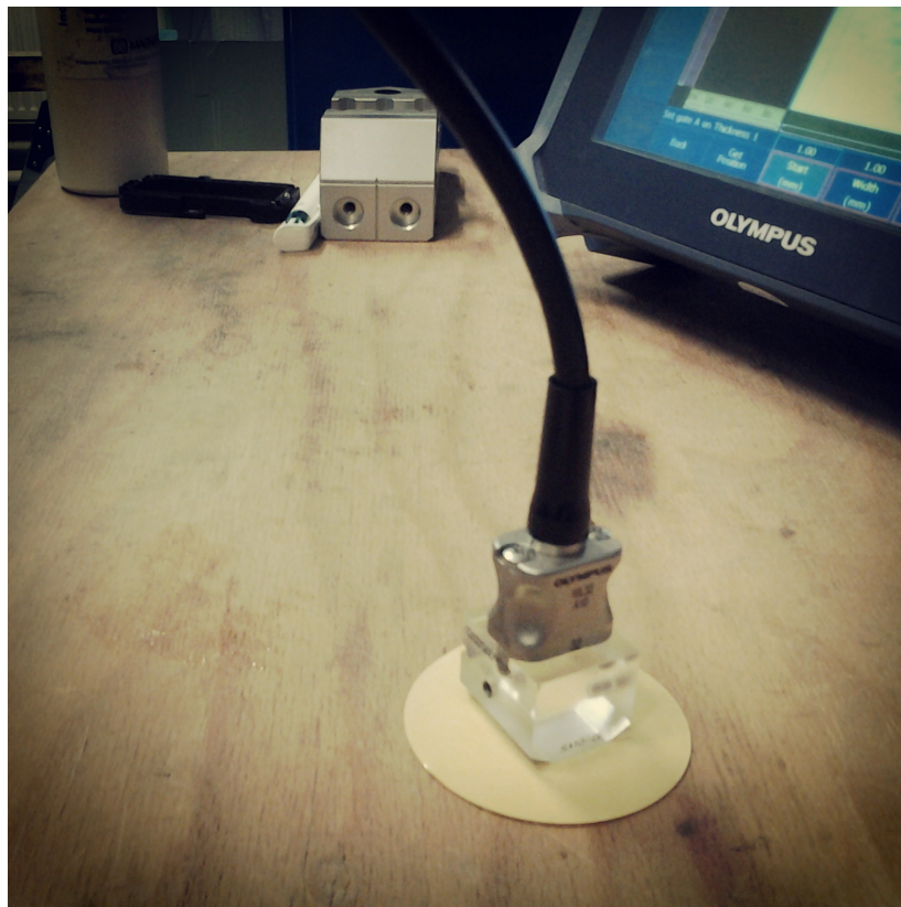
Figure 4.5.2: The sample, wedge connected to setup for measurement.
