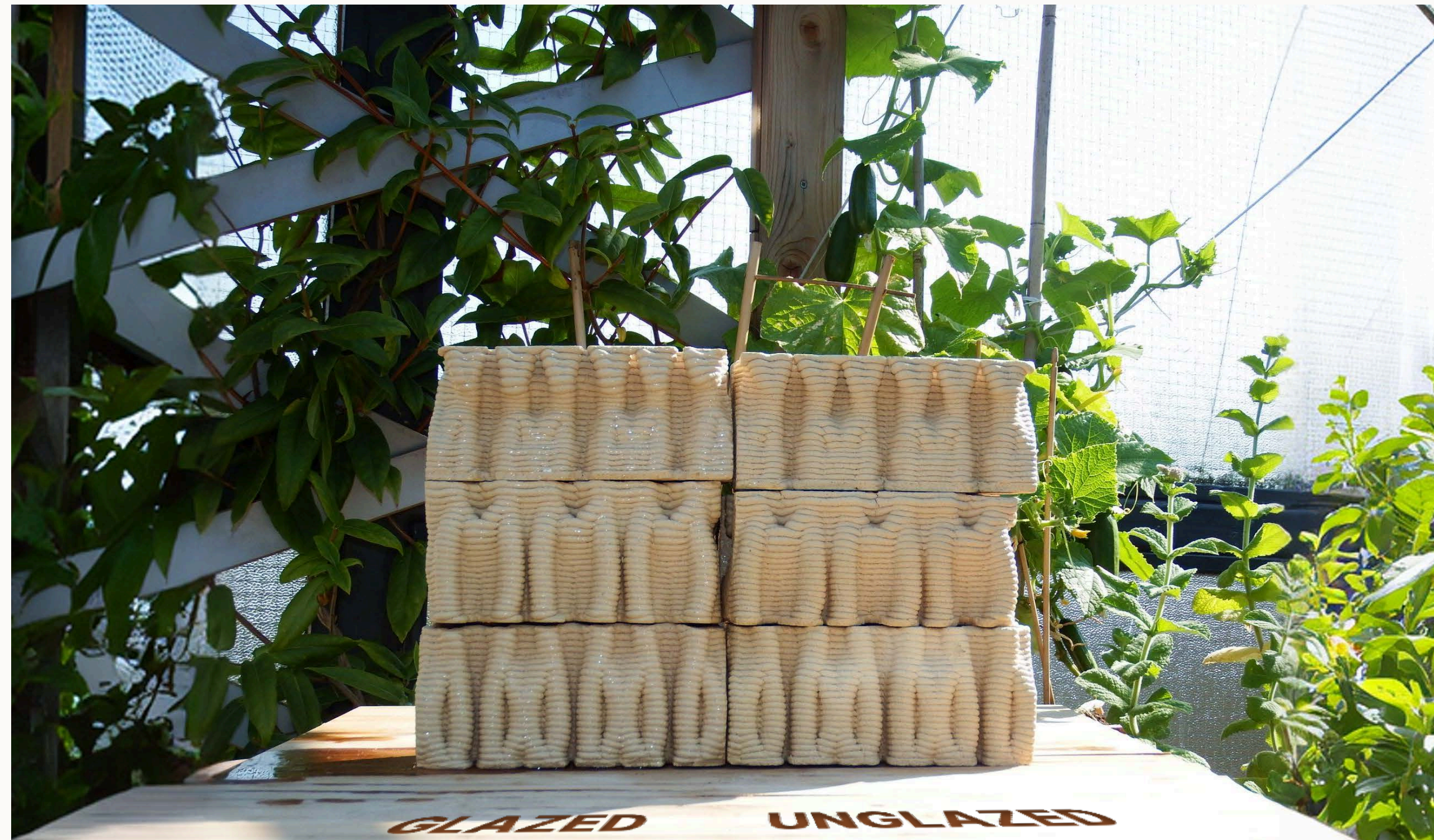
Fig. 5.8 — Cooling experiment set-up, glazed v.s. unglazed ceramic modules
