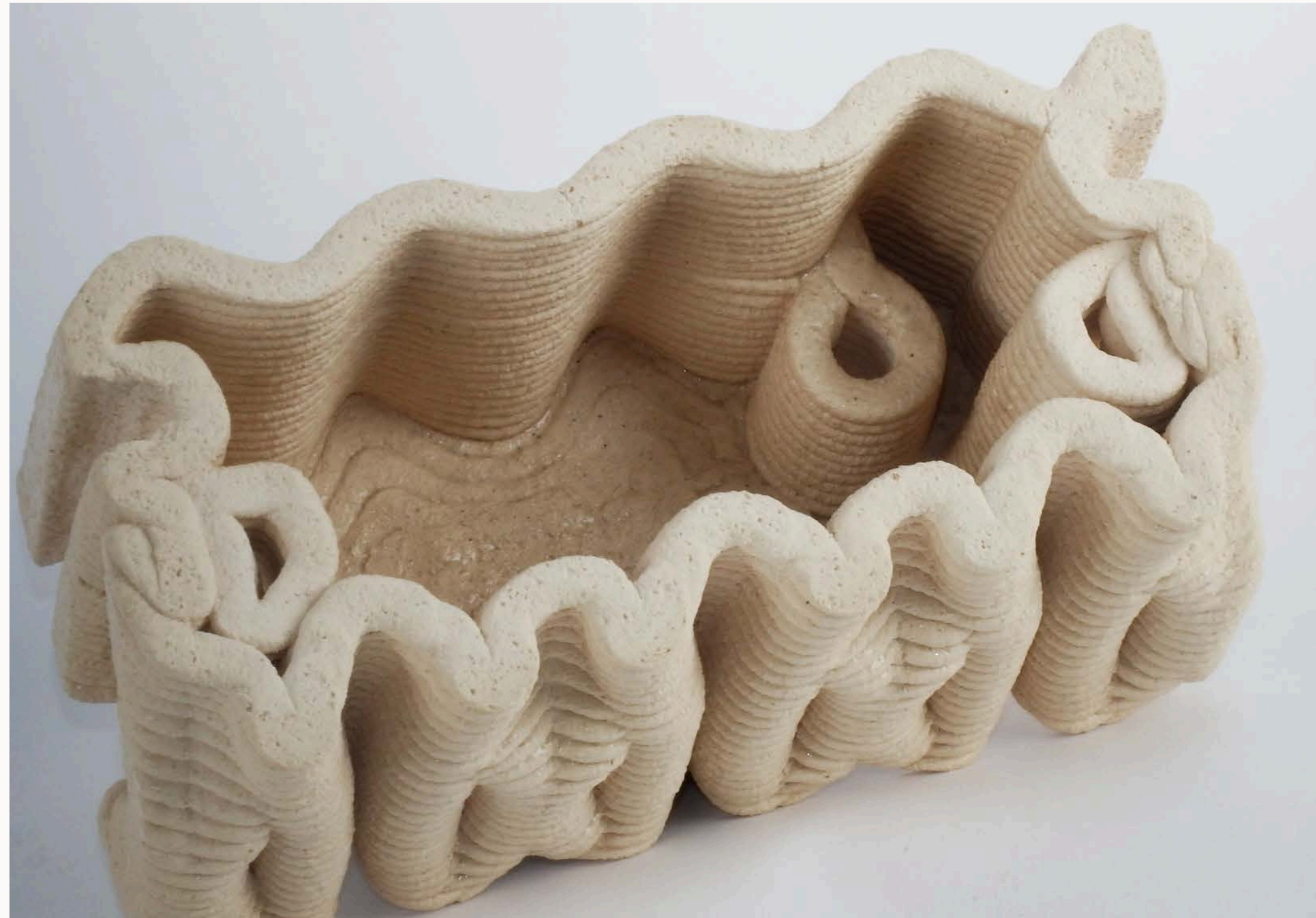
Fig. 5.2 — Internal Cavity of the 3D-Printed Ceramic Tile Functioning as a Rainwater Storage and Buffering Basin
