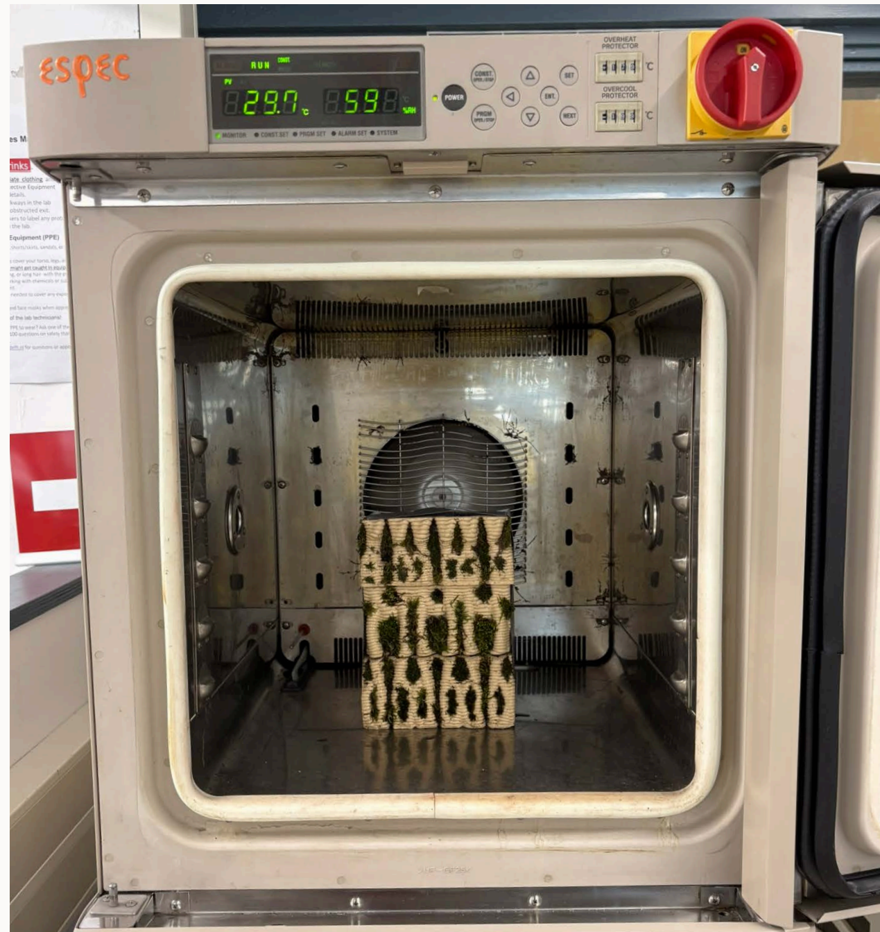
Fig. 5.26 — Climate-chamber set-up: the saturated glazed-moss module dried at a constant 30 °C and 60 % RH.
