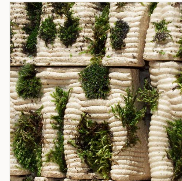
Fig. 5.18 — Moss attached on the ceramic tiles using the moss slurry as glue
