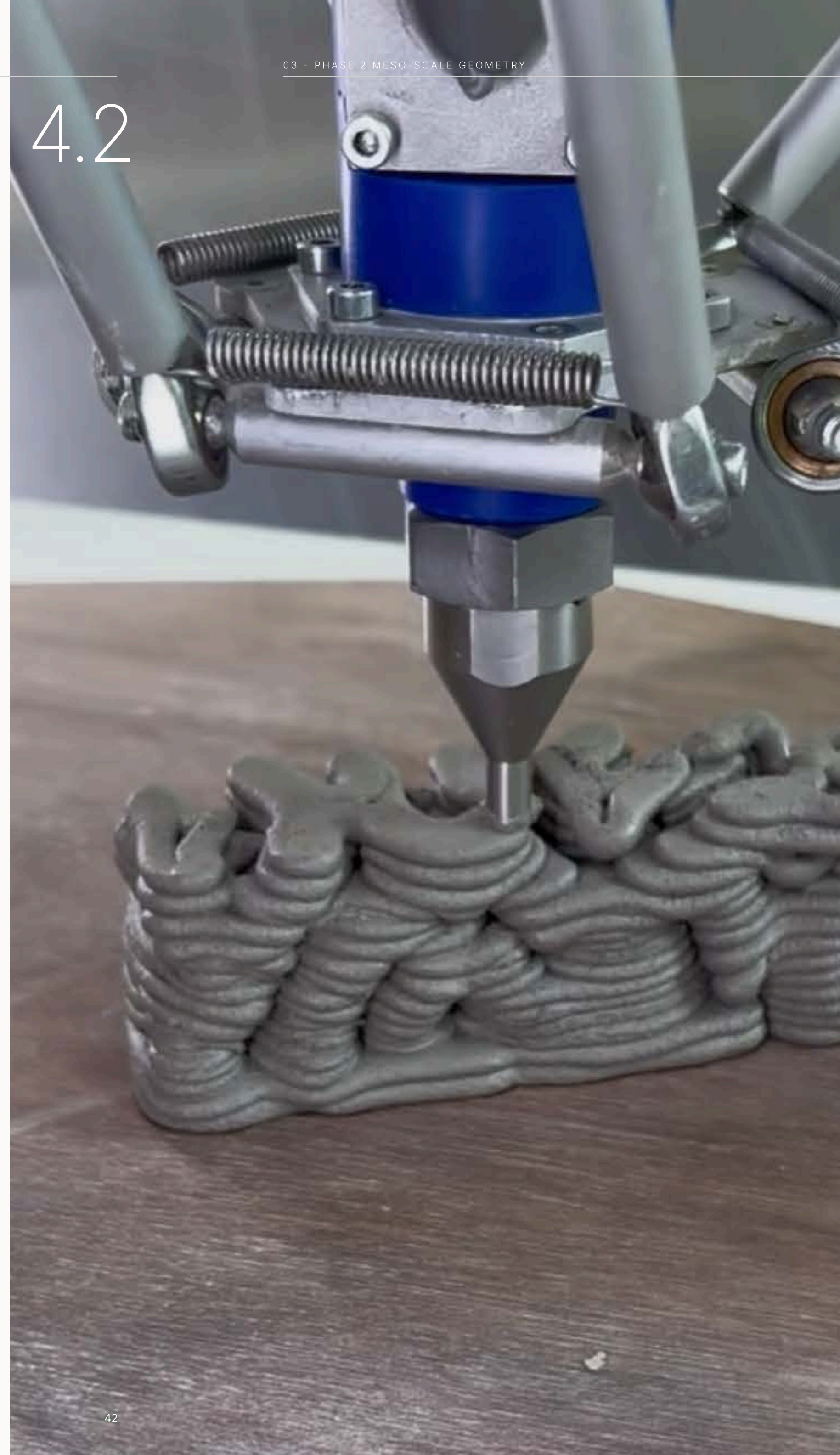
Fig. 4.2 — Liquid Deposition Modeling: ceramic paste extruded layer by layer through the nozzle to form the printed tile.
