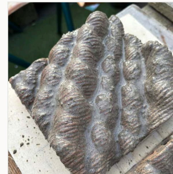
Fig. 5.17 — Moss slurry applied on fired ceramic
