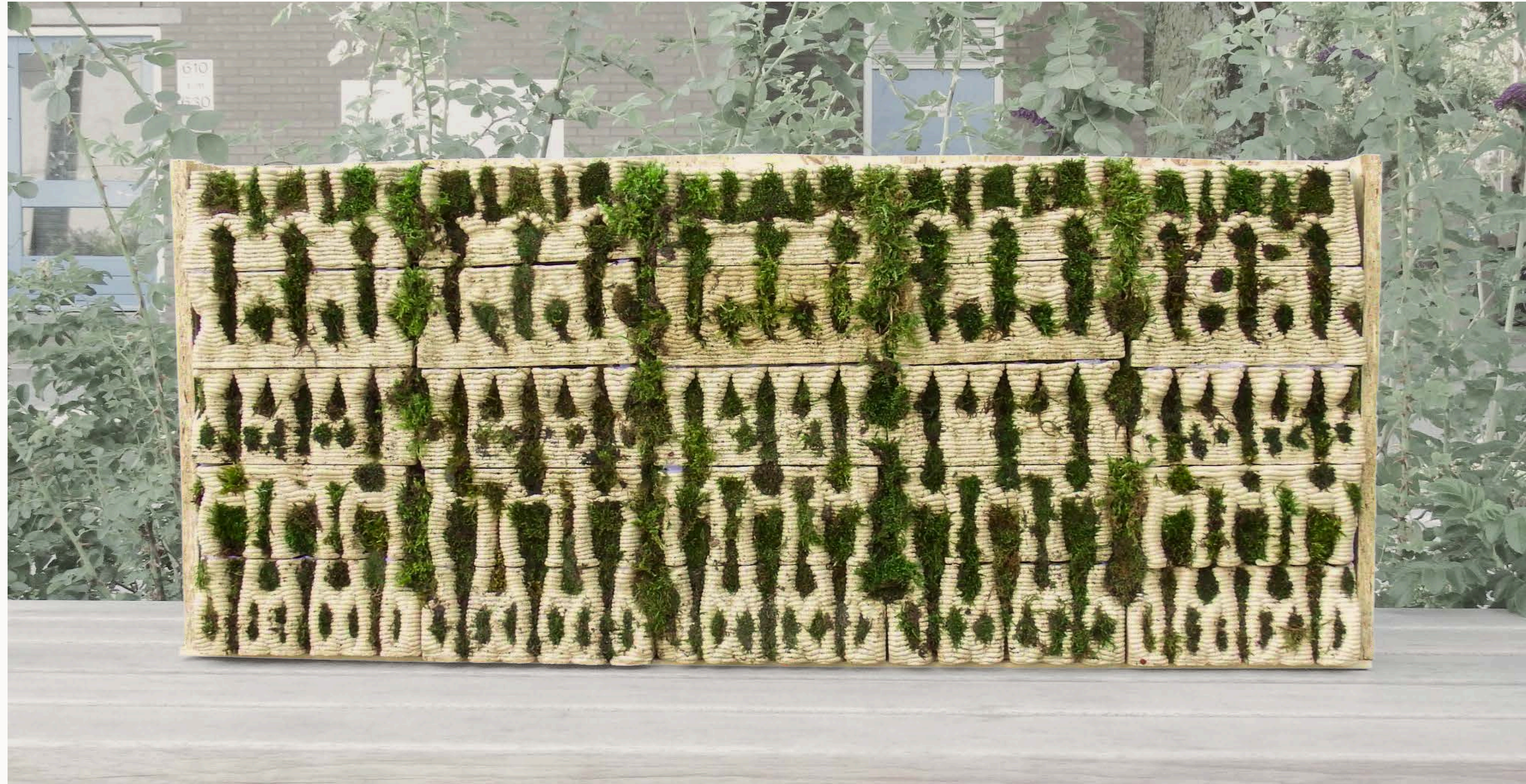
Fig. 6.2 — The prototype with its living layer: moss transplanted into the printed channels of the 3D-printed ceramic facade.
