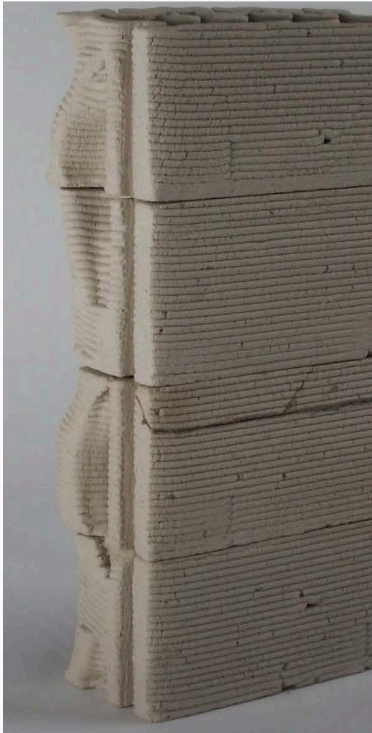
Fig. 5.4 — Printed column module.
