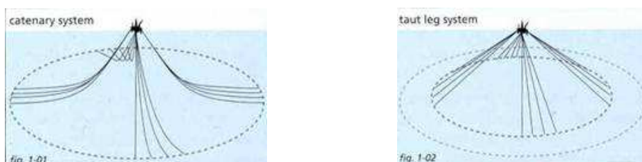
Figure 8.7 Seafloor footprint of a catenary mooring (left) and a taut line mooring (right) 4
