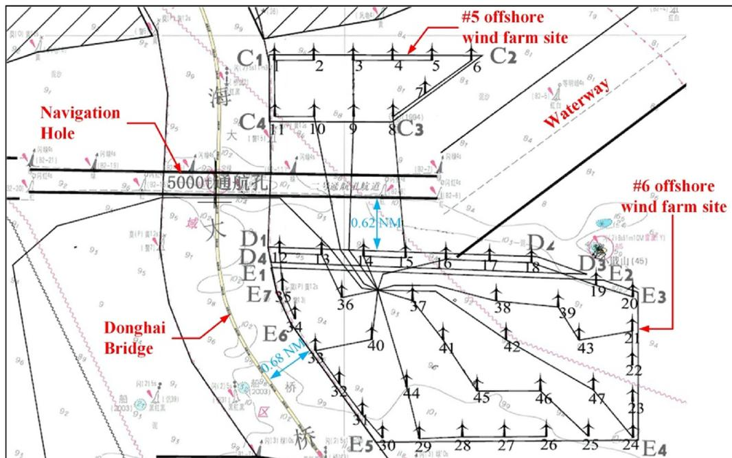
Fig. 8. An alternative construction plan for the 6 MW offshore wind turbines.
