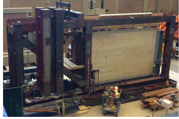
Figure 3: Setup for in-plane tests on timber diaphragms
