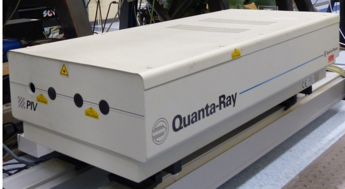
Figure 3.9: Spectral Physics Quanta-Ray, Nd: YAG laser used for the tomographic-PIV experiments.
