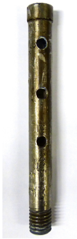
Figure A.1: Seeding tube used earlier as the seeding distribution device
