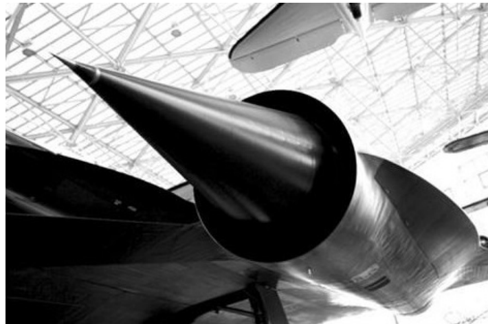
Figure 1.1: Inlet spike of a Pratt & Whitney J-58 engine used on the SR-71 Blackbird [2].
