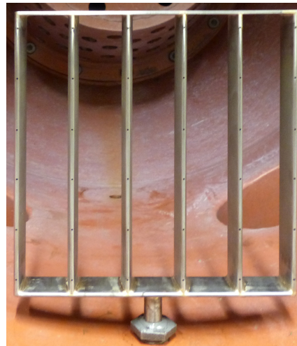
Figure A.2: Seeding Rake mounted inside the settling chamber of ST-15 wind tunnel.
