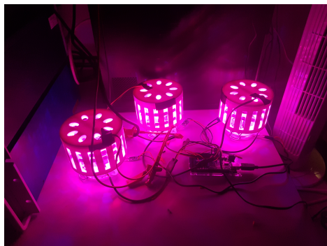
Figure C.11: Fifth setup to measure \text{CO}_2 , humidity, temperature and light in three jars simultaneously.
