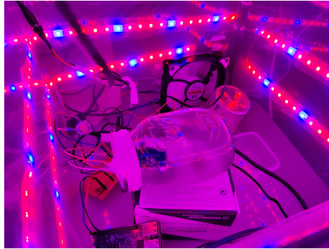
Figure C.3: Second setup to measure CO 2 , O 2 , humidity, temperature and light.
