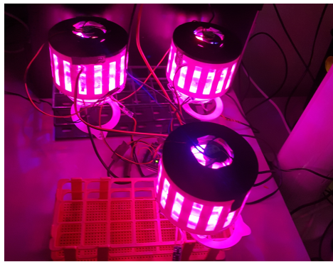
Figure C.14: Fifth setup to measure CO 2 , humidity, temperature and light in three jars simultaneously, each with its separate climate control fan.
