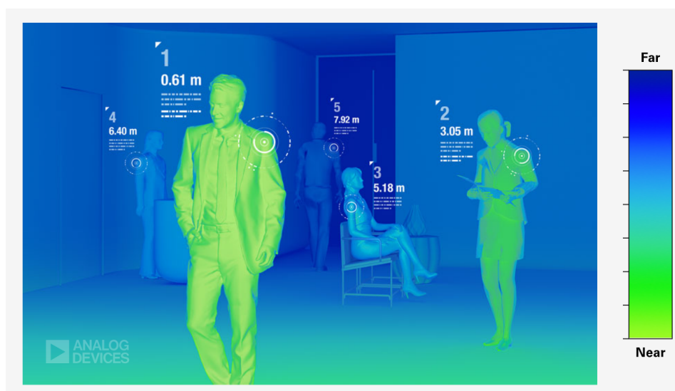
Figure 1.1: Example image of using time of flight measurement for people classification and range detection [6].
