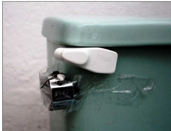
Figure 5.3-Picture of hand counter installed on toilets
