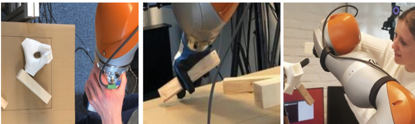
Fig. 3. Automated and HRI-supported assembly sequence relying on CV to pick-and-place linear subcomponents into the designated node.
