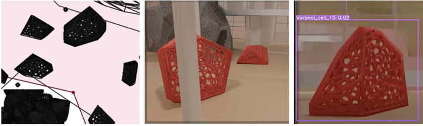
Fig. 6. Random camera and components distribution within the 3D model of library top view (left), input image from the setting (middle), and object recognition with 0.92 confidence level (right).
